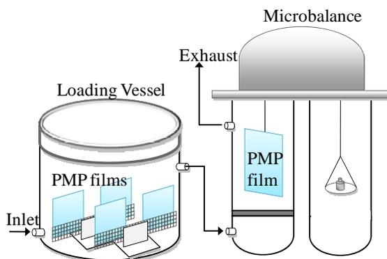
Once loaded to equilibrium, the polymer films were wrapped tightly in aluminum foil and sealed in a plastic specimen bag. The packaged films were immediately placed in a cooler containing dry ice. Dry ice was found to be necessary to keep the toluene from escaping the loaded film. Packaged films were distributed to test laboratories using coolers and dry ice. Upon receipt, laboratories were instructed to place packaged films in a laboratory freezer (-20 °C) until ready for testing.
