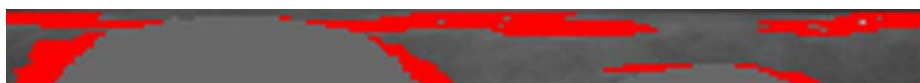
Fig. 31. Mask-if-close-and-far: VASIR's approach of masking out pixels with small magnitude values (a) masked the pixels with a magnitude below 1% and above 80% (see red area).
