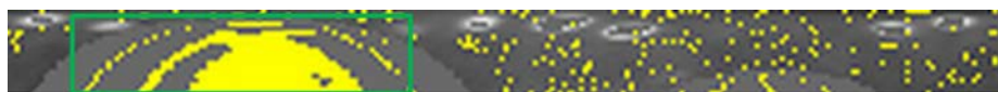
Fig. 30. Mask-if-fragile: Hollingsworth's approach of masking out the pixel of “fragile bits” where bits are near to either the real axis or the imaginary axis (masked out 10% of fragile bits—see yellow area).
