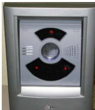
Fig. 2. A LG2200 System with three LED illuminators—taken from the paper written by Bowyer and Flynn [11] with permission.
