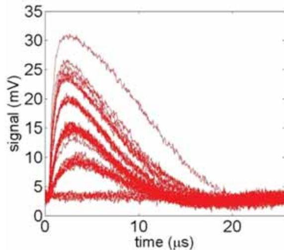
Figure 2: Electrical TES output traces for different numbers of photons in the weak laser pulse; the photon number resolving capability is clearly visible here
