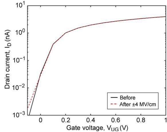
Fig. 4. Turn-on characteristics, i.e., drain current as a function of gate voltage of a MOSFET transistor with 25 nm gate oxide thickness. Data were taken with the drain voltage  $V_D$  of 1 mV. Solid (black) line is initial turn-on curve, and dashed (red or gray) line is turn-on curve after  $\pm 10$  V (4 MV/cm) excursion in the gate voltage. The identical curves indicate immunity to dielectric breakdown up to  $\pm 4$  MV/cm.
