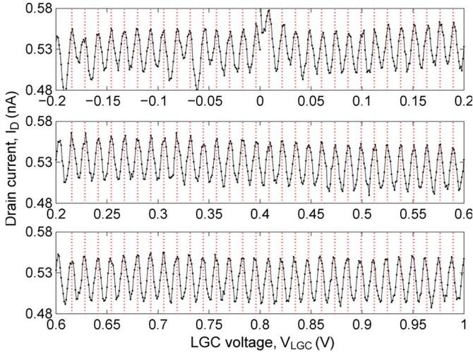
Fig. 5. SET oscillations of a device at 2.2 K; vertical dashed lines (red or gray) are separated by a period of 12.9 mV. The data show good uniformity of the gate capacitance over 90 periods.
