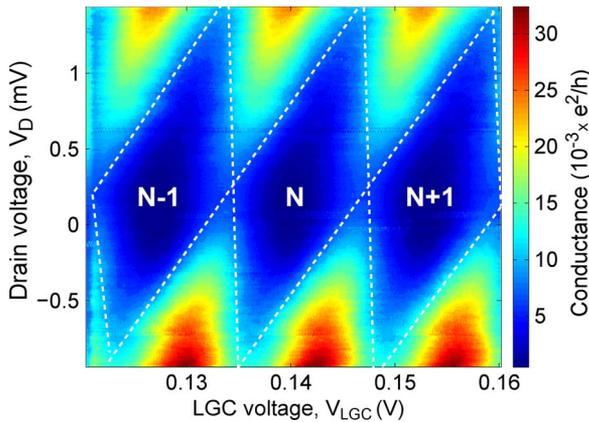
Fig. 6. Coulomb diamonds measured at 30 mK for a SET device;  $N$  is the electron number. Charging energy  $E_C = 1.2$  meV, drain capacitance  $C_D = 7$  aF, and total capacitance of the island  $C_\Sigma = 70$  aF, extracted from the diamond data.
