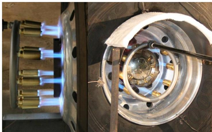
Figure 2 (Left) A photograph showing the burner pre-mixed natural gas and air torches impinging on a tag axle wheel. (Right) A photograph showing the tire shield inside a drive axle wheel rim with an insulating cover to minimize heating from the shield to the tire.
