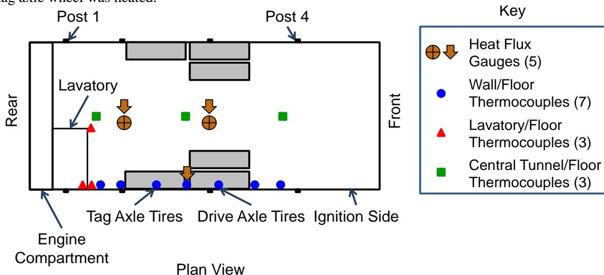
Figure 3 A diagram of the motorcoach showing locations of interior floor thermocouples and the locations and directions of heat flux gauges for penetration and hardening tests.
