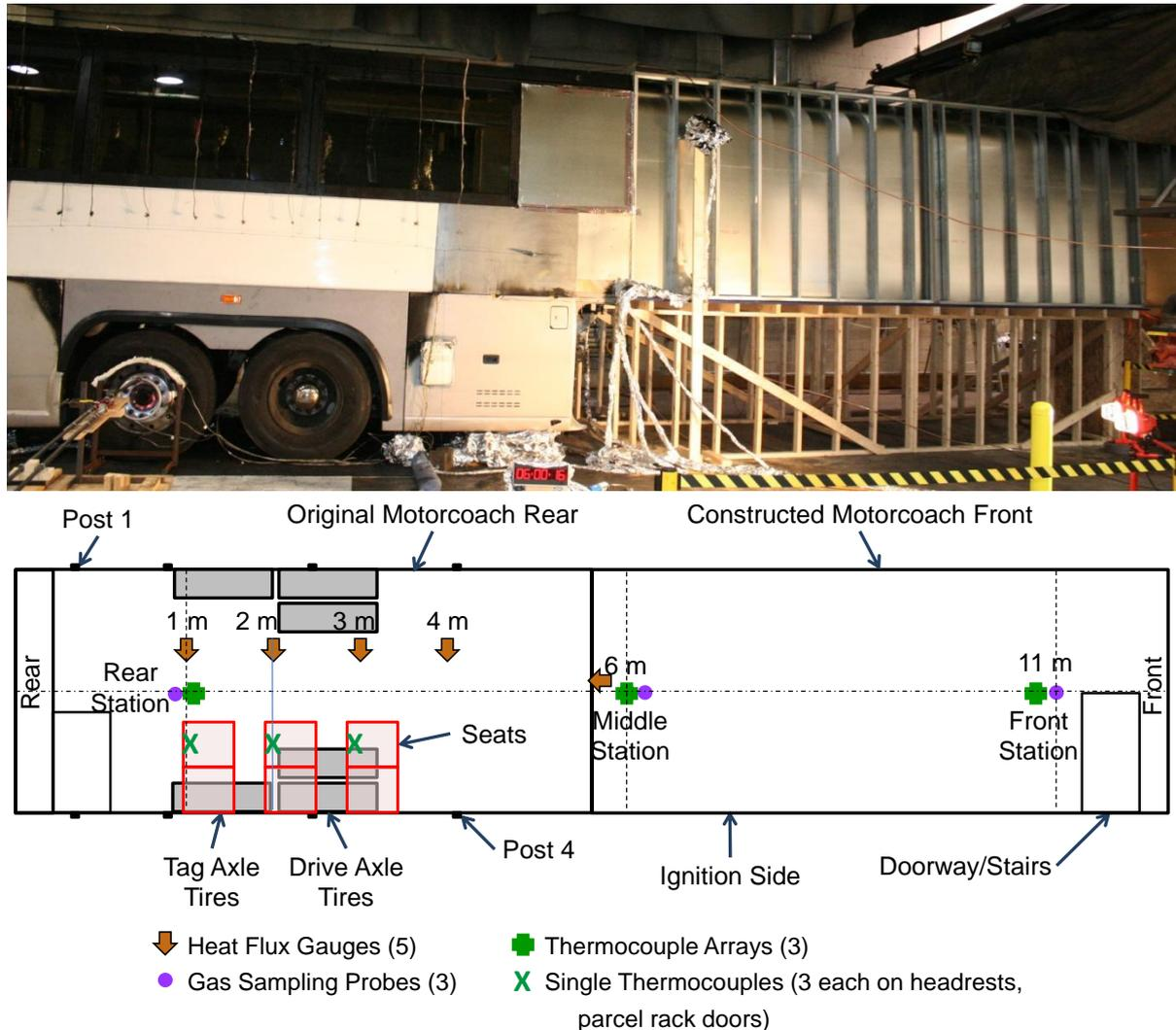
Figure 6 (Top) Photograph showing the assembly of the original motorcoach rear half and added front. (Bottom) Diagram showing the layout of measurements for the tenability test.
