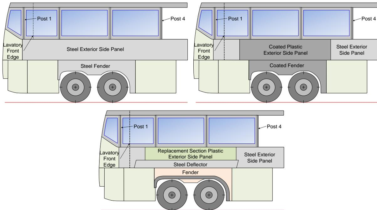
Figure 4 Diagrams of the right side of the motorcoach showing the three fire hardening configurations: steel exterior side panel and fender (upper left); intumescent coating on panel and fender (upper right); steel deflector between the fender and panel (bottom).
