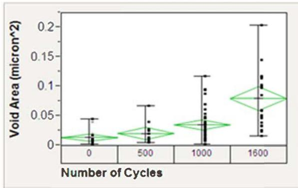
Figure 3: Plot of the void area in SiO<sub>2</sub> isolation layer as a function of the number of thermal cycles.
