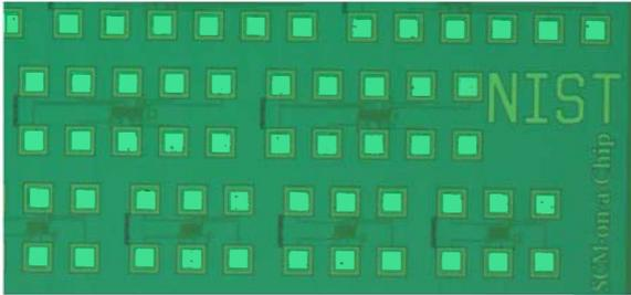
Figure 4: CBCM measurement circuits with various on-chip compensation capacitors.
