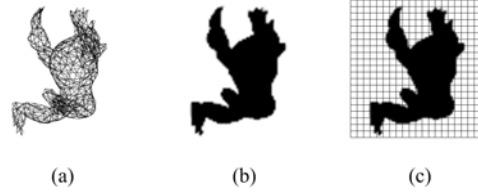
Figure 6. A 2D projection of a 3D mesh. (a) is the exact shape of the projection while (b) is the silhouette view. Based on the number of black pixels in (c), area of the projected shape can be estimated.
