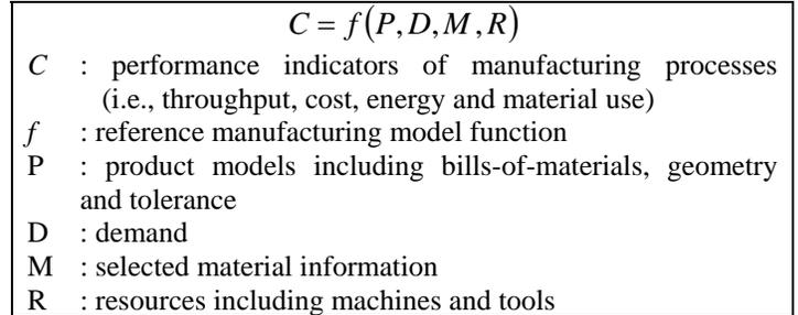
Figure 4 Function between manufacturing process information and performance
