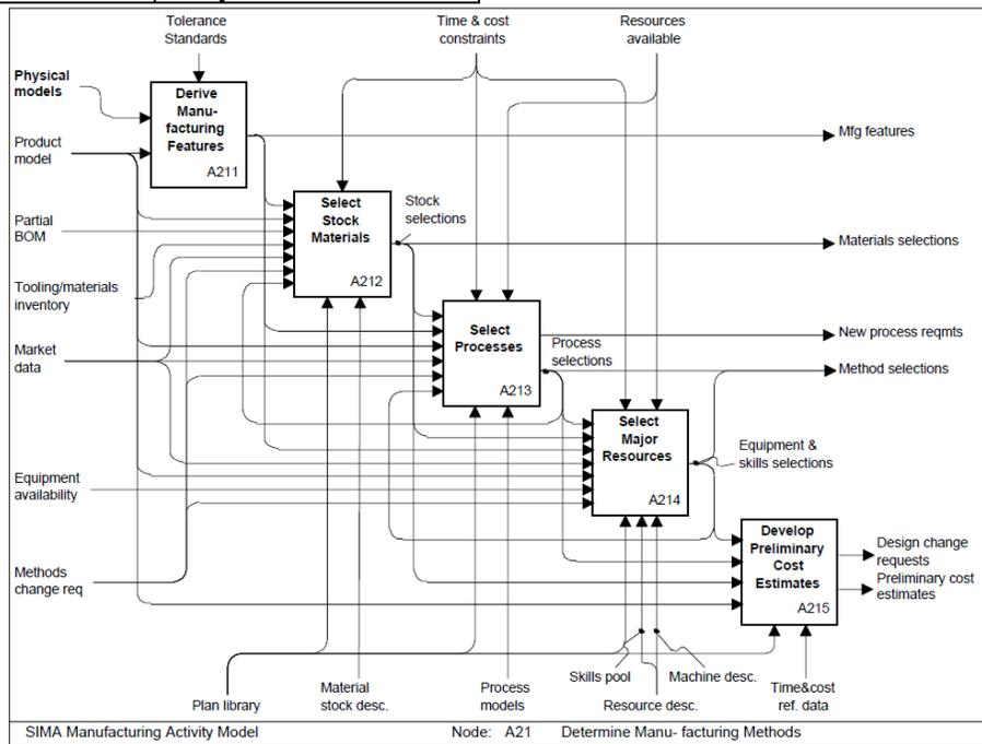
**Figure 2** SIMA model: A21 Activity Model- Determine manufacturing methods
