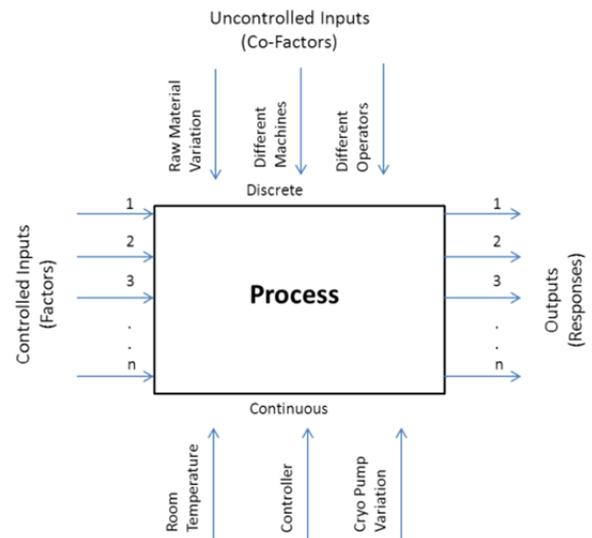
Figure 1 Boundaries of a process under study [7]
