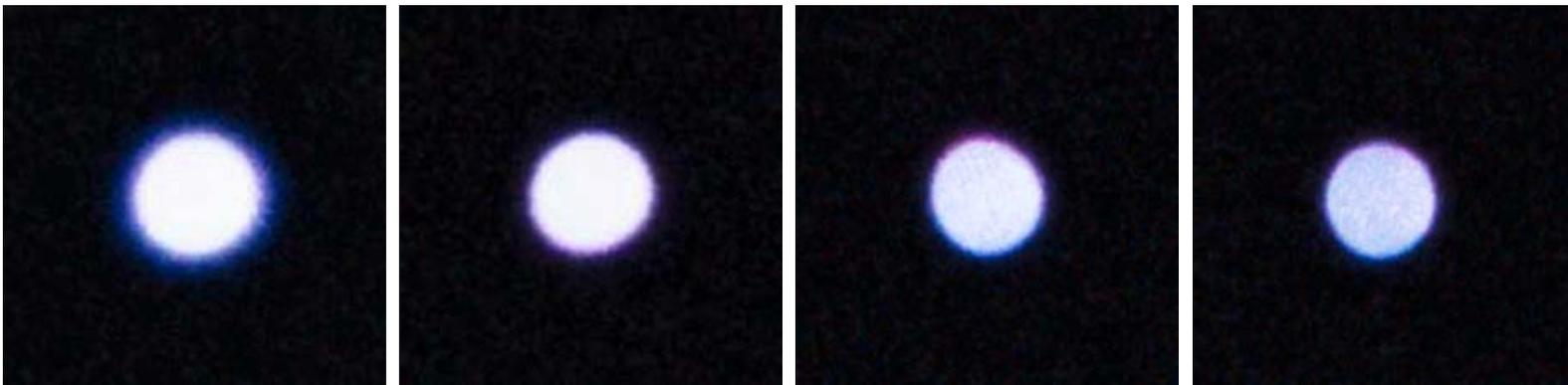
**Figure 27.** Effect of f# on droplet images. 2800  $\mu\text{m}$  diameter water drops with approximately 3 mg/L of stilbene and 3.3 mg/L of rhodamine illuminated with 355 nm laser sheet. Image quality improves as f# is increased from 2.8 to 8.0 as evidenced by haze around droplet perimeter. Images taken at f#s of 5.6 and 8.0 are of nearly equal quality.
