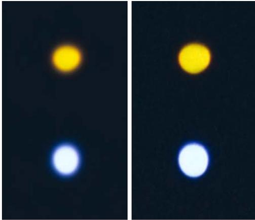
**Figure 28.** Effect of scanner focus on droplet images. The images in this figure show nominally 3000  $\mu\text{m}$  diameter droplets illuminated with 532 nm (upper drops) and 355 nm (lower drops) laser sheets. The images are two successive scans of the same film. Care must be taken to verify that the scanner is properly focused, a procedure that is important with small pixel sizes.
