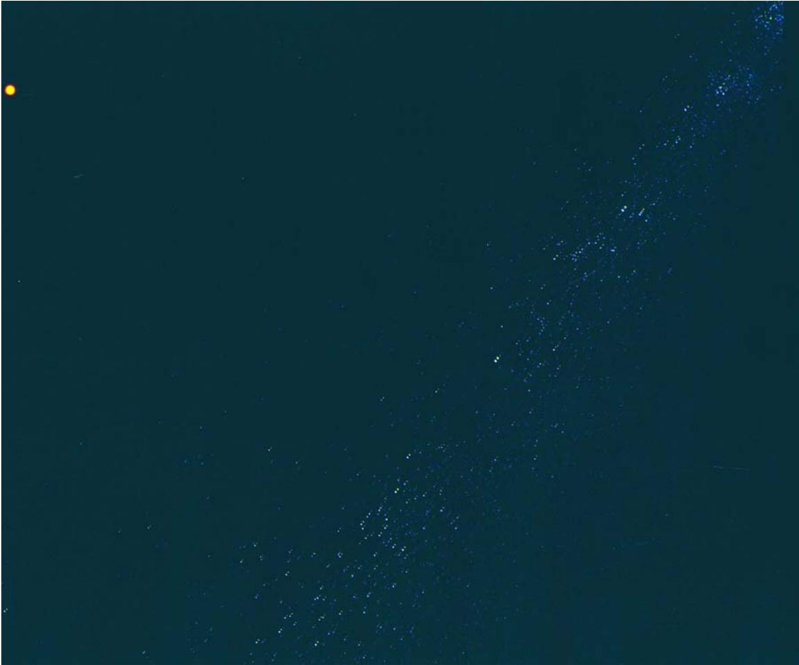
**Figure 50.** Axis-symmetrical sprinkler with 4 mm nominal diameter orifice and 90 degree strike plate operating at approximately 6 gpm. Image area is approximately 21 inches wide by 17 inches high. The upper right hand corner of the image area is located approximately 6 inches vertically down from the orifice, and 5 inches horizontally from the symmetric centerline of the orifice. The large orange circle is a light emitting diode used as a reference location
