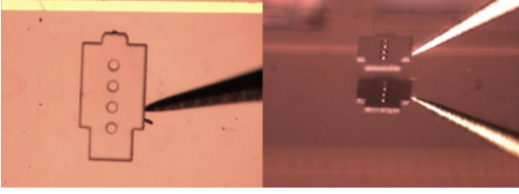
Fig. 4. Part supported by a single probe.
