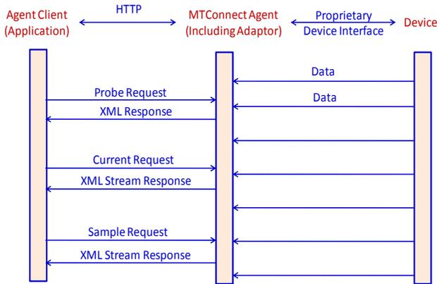
Figure 3 - MTCConnect Communication Protocol
