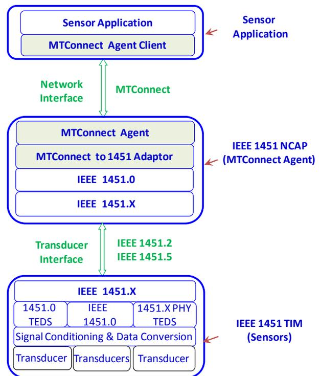
Figure 6 - Integration architecture of MTConnect with IEEE 1451 sensor networks
