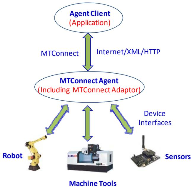
Figure 1 - Architecture of MTConnect
