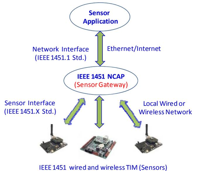
Figure 2 - Architecture of IEEE 1451 standard-based sensor networks
