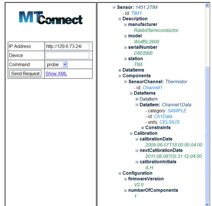
Figure 11 - Screenshot of a Probe request of a MTConnect Agent Client
