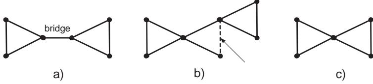
Figure 9: Examples of simple graphs that are not 2-vertex connected.
