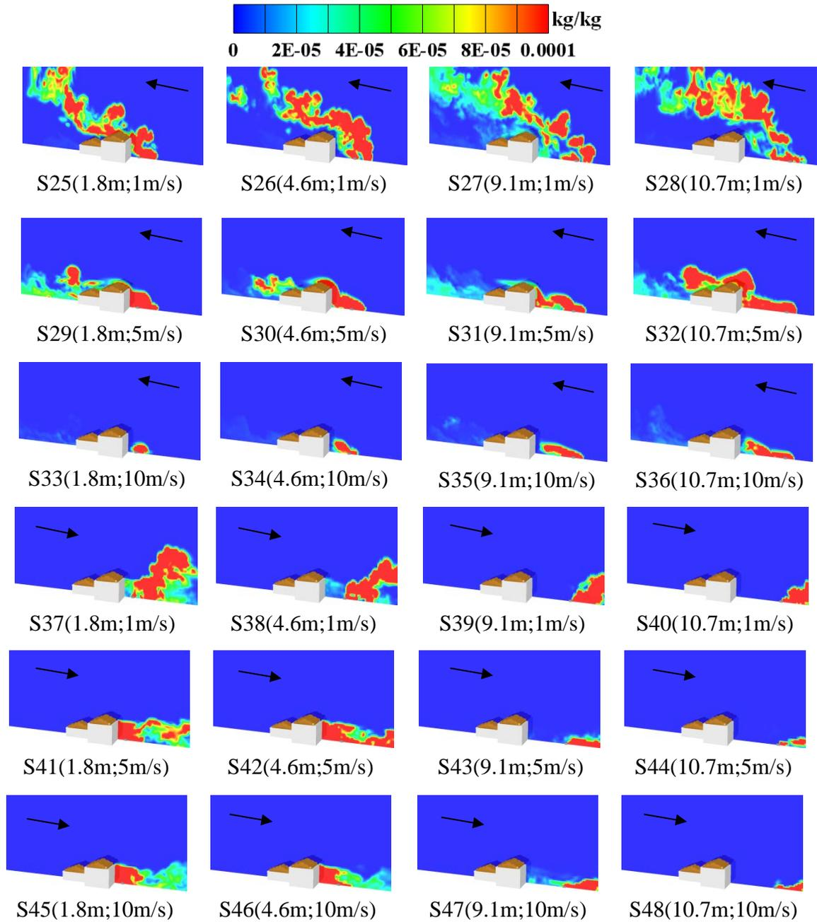
Figure 6. Comparison of CO levels at the middle lengthwise plane of the house for different generator distance, location, wind direction and speed when the generator exhaust pointed away from the house.
