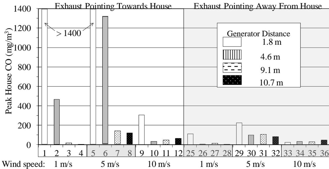
Figure 8. Maximum indoor CO in the house when the generator was operating upwind of the house for 8 hours under zero indoor and outdoor temperature difference.
