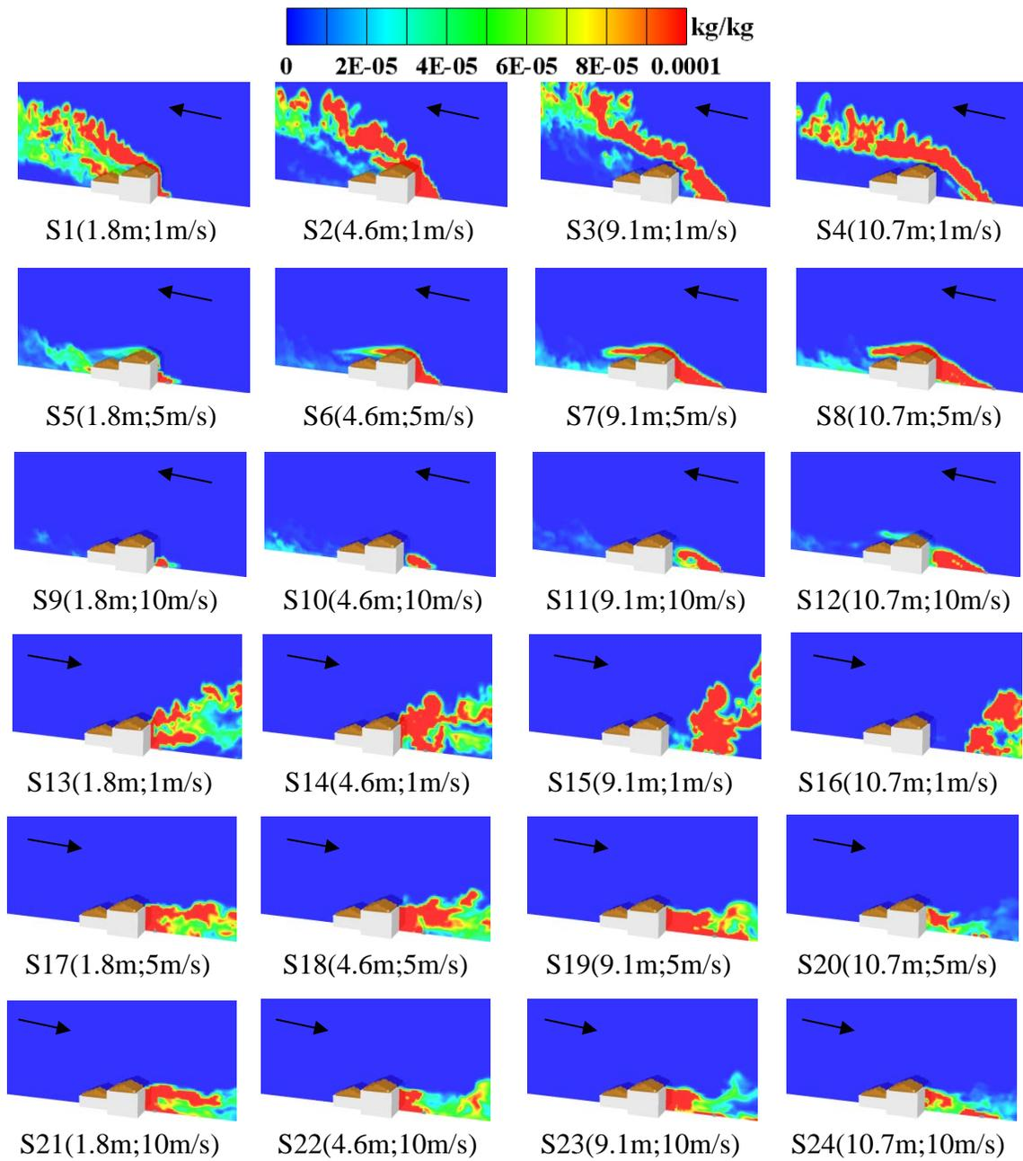
Figure 5. Comparison of CO levels at the middle lengthwise plane of the house for different generator distance, location, wind direction and speed when the generator exhaust pointed towards the house (for CO in air,  $1.0 \text{ kg/kg} \approx 1.2 \times 10^6 \text{ mg/m}^3$  at  $20.9^\circ\text{C}$  and  $101.325 \text{ kPa}$ ).
