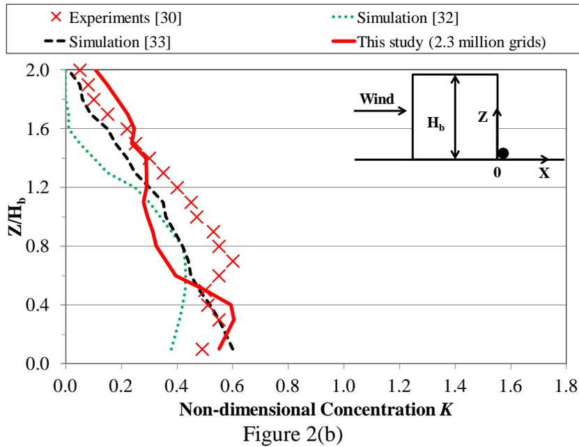
Figure 2. (a) Non-dimensional concentrations in the lateral direction at  $Z/H_b = 0$  and (b) in the vertical direction along the centre line at  $X/H_b = 3$ , when the tracer source is located at the ground corner of the building.
