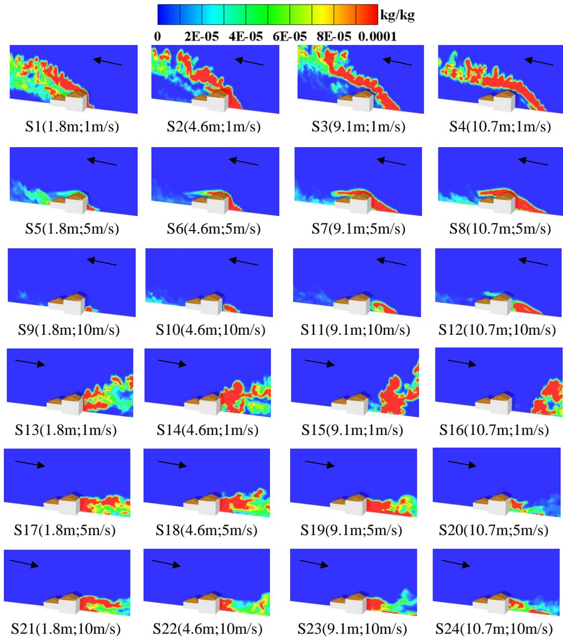
Figure 5. Comparison of CO levels at the middle lengthwise plane of the house for different generator distance, location, wind direction and speed when the generator exhaust pointed towards the house (for CO in air,  $1.0 \text{ kg/kg} \approx 1.2 \times 10^6 \text{ mg/m}^3$  at  $20.9^\circ\text{C}$  and  $101.325 \text{ kPa}$ ).
