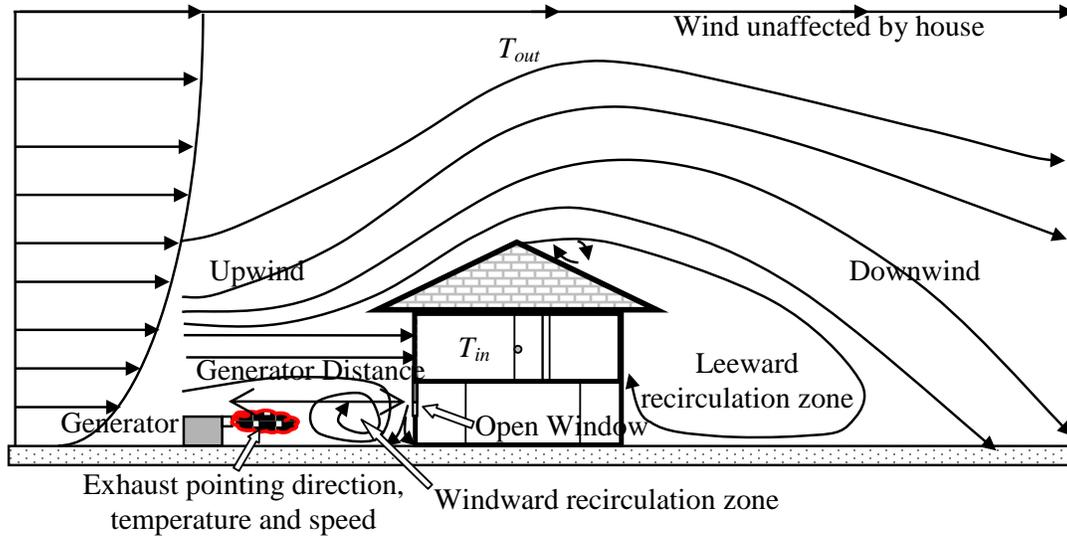
Figure 1. Schematic of airflow streamlines and factors affecting house CO entry when a generator is placed upwind of a two-story house and the exhaust is pointed towards the house.
