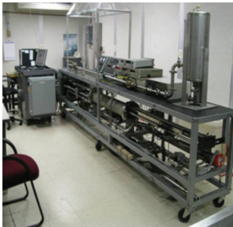
Figure 1. The NIST 20 L piston prover. Flow directions in the schematic are shown for the piston travelling from left to right. The T and P symbols represent temperature and pressure sensors.
