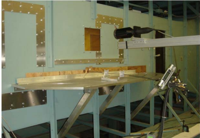
FIGURE 1. Manual 3-D calibration rig.
