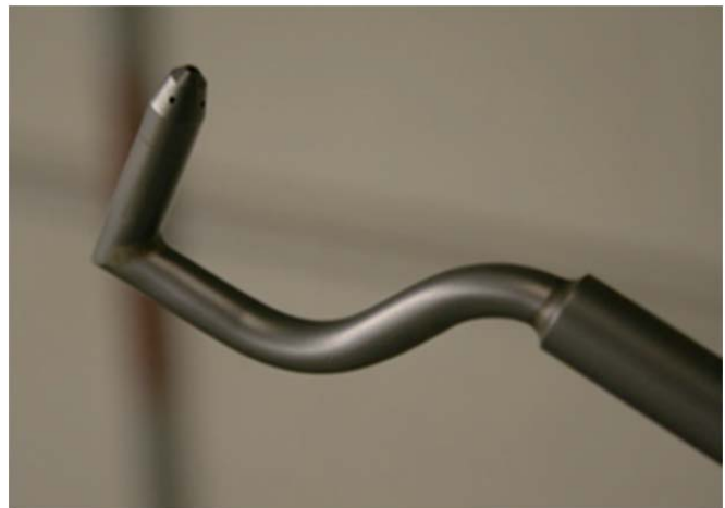
Figure 2. Cone-shaped, five-hole pitot tube. The diameter of the curved tube was 9.5 mm.
