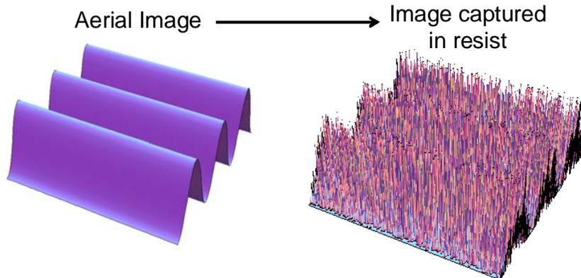
Figure 1: Illustration of the effect of wave function collapse, i.e., exposure statistics. On the left is a 50 nm period sinusoidal aerial image intensity, plotted, as usual, as a smooth continuous surface. On the right is the result of exposing that aerial image in resist. The Poisson statistics (discussed in the text) used to generate the plot on the right assumed a pixel size of  $1 \text{ nm}^2$  and the exposure dose corresponded to  $5 \text{ mJ/cm}^2$ .
