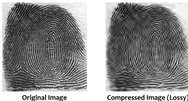
Figure 1 - Example of Fidelity Degradation Due to Extreme Lossy Compression (JPEG 2000 at 800:1)
