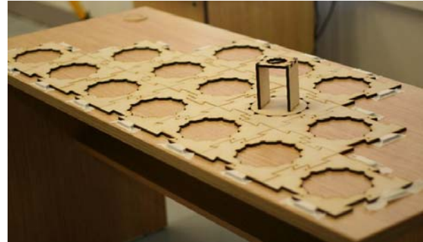
Figure 6. The GT2012 fixture configured for measurement accuracy testing. The base platform can be expanded by attaching additional plates via side interlocks.
