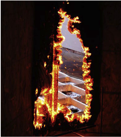
Fig. 3. Picture of flaming re-entrant corner assembly at 6 m/s wind speed (Experiment No. 2).
