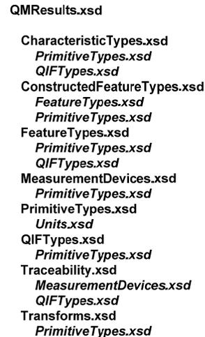
Fig. 1 Structure of QMResults.xsd
