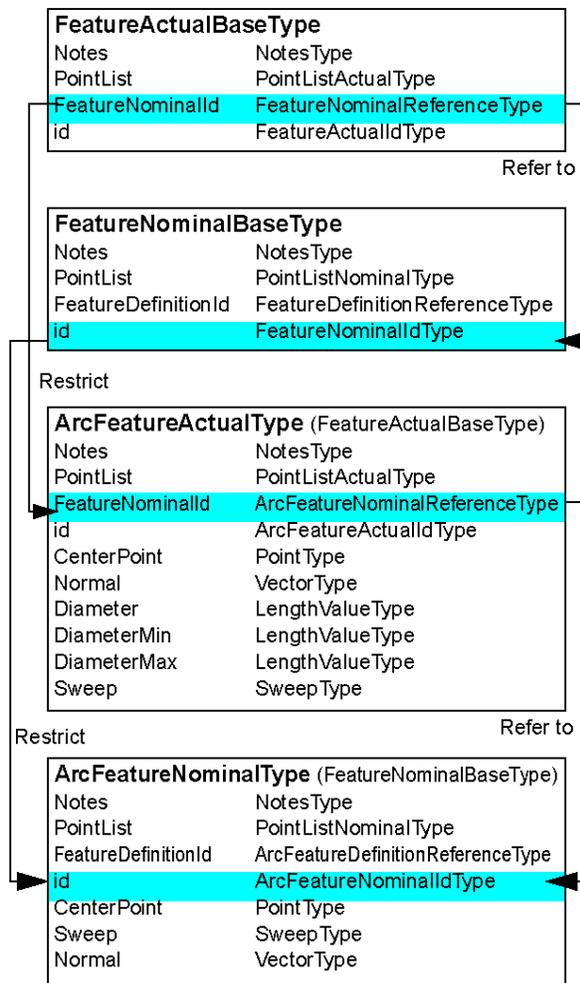
**Fig. 6 Semantic connection between feature actual and feature nominal, specialized to the connection between arc feature actual and arc feature nominal**
