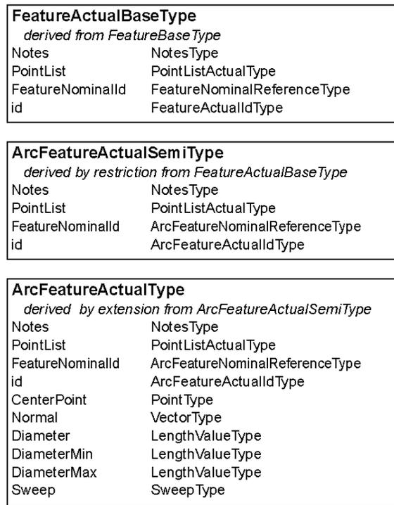
**Fig. 7 Derivation of Types in Two Stages**
