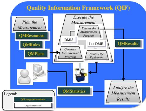
**Fig. 1 A quality measurement activity diagram with QIF application area standards (black boxes).**
