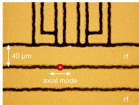
FIG. 1 (color online). Micrograph of ion-trap electrodes. The radio-frequency (rf) and static-potential electrodes are microfabricated using a 10- $\mu\text{m}$ -thick, electroplated Au film with 5- $\mu\text{m}$  gaps between the electrodes (darker areas). The red dot represents the location of the ion.
