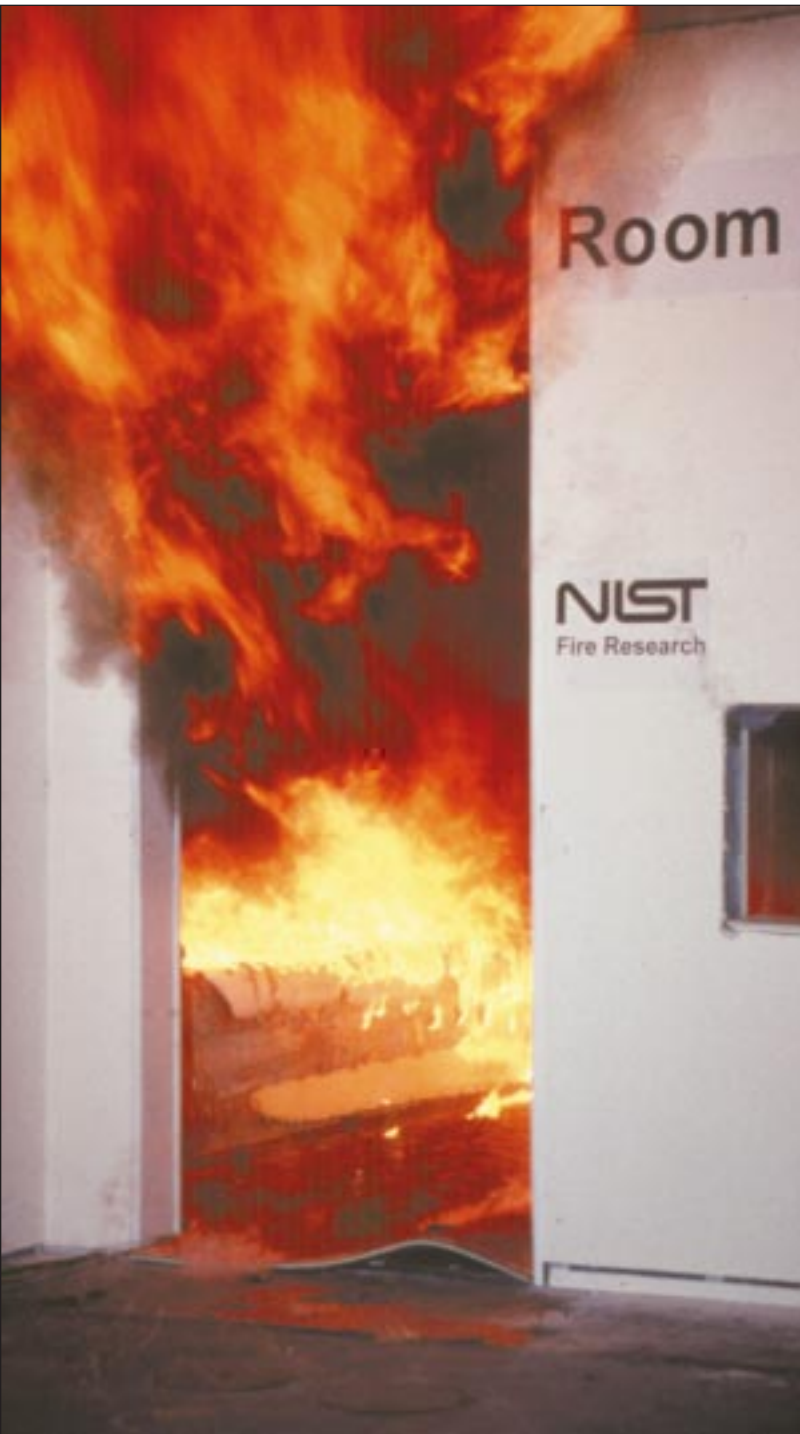
Part of a series of flashover fire tests conducted by NIST.
