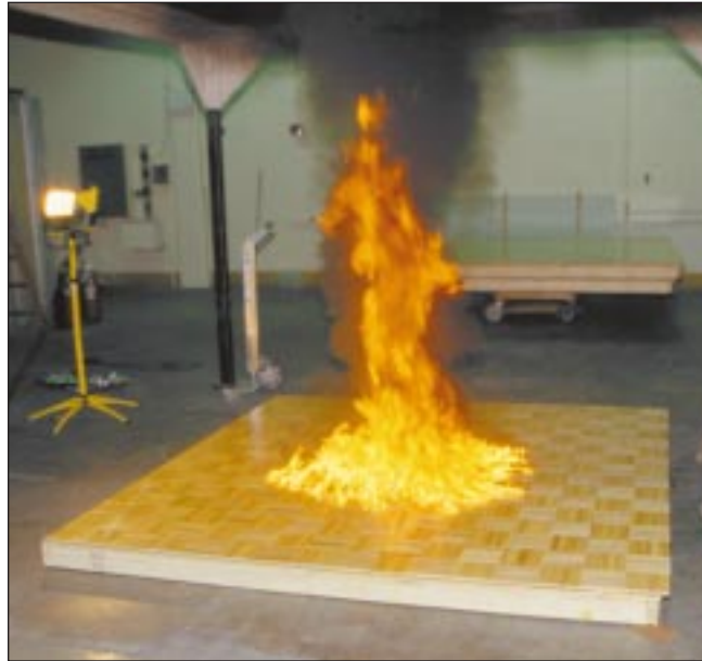
A parquet floor burns during the NIST liquid fuel spill burn pattern study.
