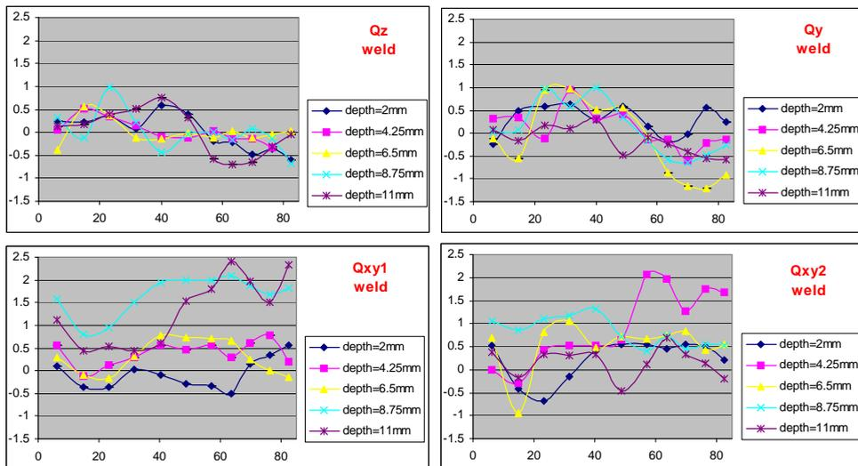
Fig. 12(a). Original strain data ( $\times 10^3 \mu$ ) for weld centerline in groove-weld segment, ( $Q_{xy1}$  and  $Q_{xy2}$  correspond to  $\varphi = \pm 42^\circ$ ; counting-statistic uncertainties are typically about  $\pm 0.035$ ; abscissa is Y-distance from flange edge (mm; beam centerline is 76.8mm)
