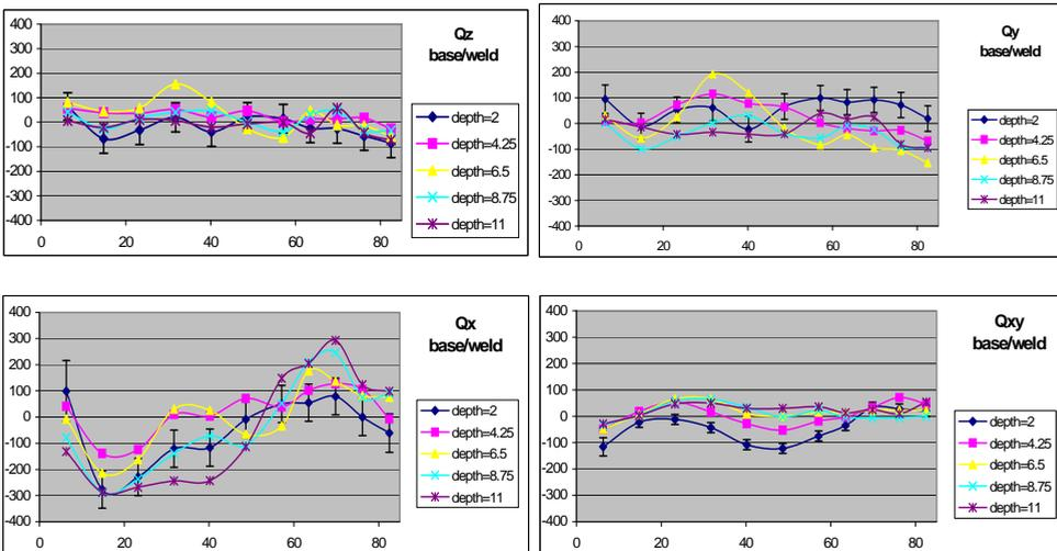
Fig. 13. Converted stress data (unit: MPa; 6.895 MPa=1ksi) for weld toe in groove-weld segment ( $Q_{xy}$  Corresponds to stress shear component. Depth unit is mm; abscissa is Y-distance from flange edge (mm; beam centerline is 76.8mm)
