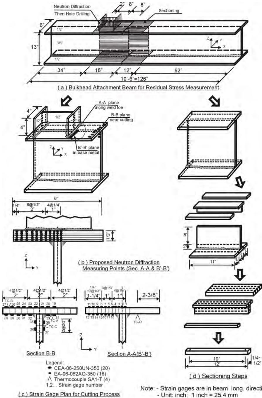
Fig. 4. Two-step residual stress measurement of attachment beam
