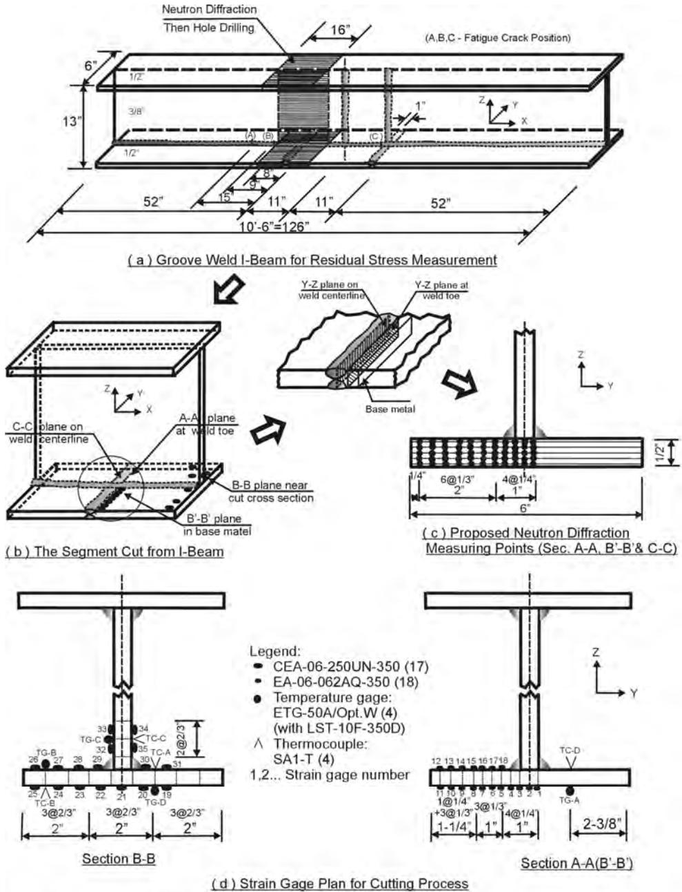
Note: - All strain gages are in the beam longitudinal direction.
