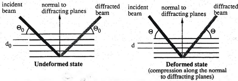
(a) Neutron Diffraction Measurement for Different Lattice Spacing
