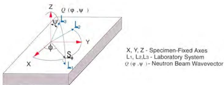
Fig. 7. Two coordinate systems for neutron diffraction measurement
