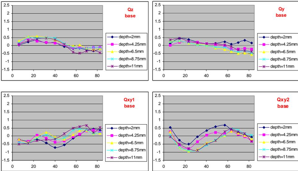
Fig. 12(c). Original strain data ( $\times 10^3$  micro-strain) for base metal in groove-weld segment ( $Q_{xy1}$  and  $Q_{xy2}$  correspond to  $\phi = \pm 42^\circ$ ); counting- statistic uncertainties are typically about  $\pm 0.035$ ; abscissa is Y-distance from flange edge (mm; beam centerline is 76.8mm)
