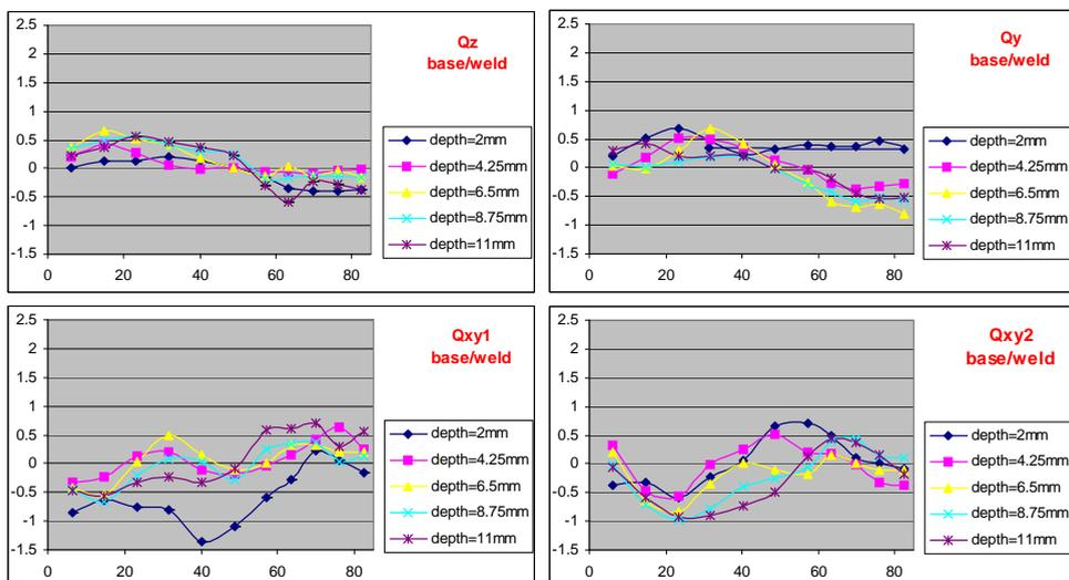
Fig. 12(b). Original strain data ( $\times 10^3$  micro-strain) for weld toe in groove-weld segment, ( $Q_{xy1}$  and  $Q_{xy2}$  correspond to  $\varphi = \pm 42^\circ$ ; counting-statistic uncertainties are typically about  $\pm 0.035$ ; abscissa is Y-distance from flange edge (mm; beam centerline is 76.8mm)
