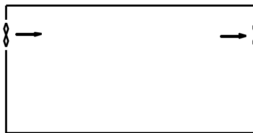
(c) Space With Cross Ventilation
