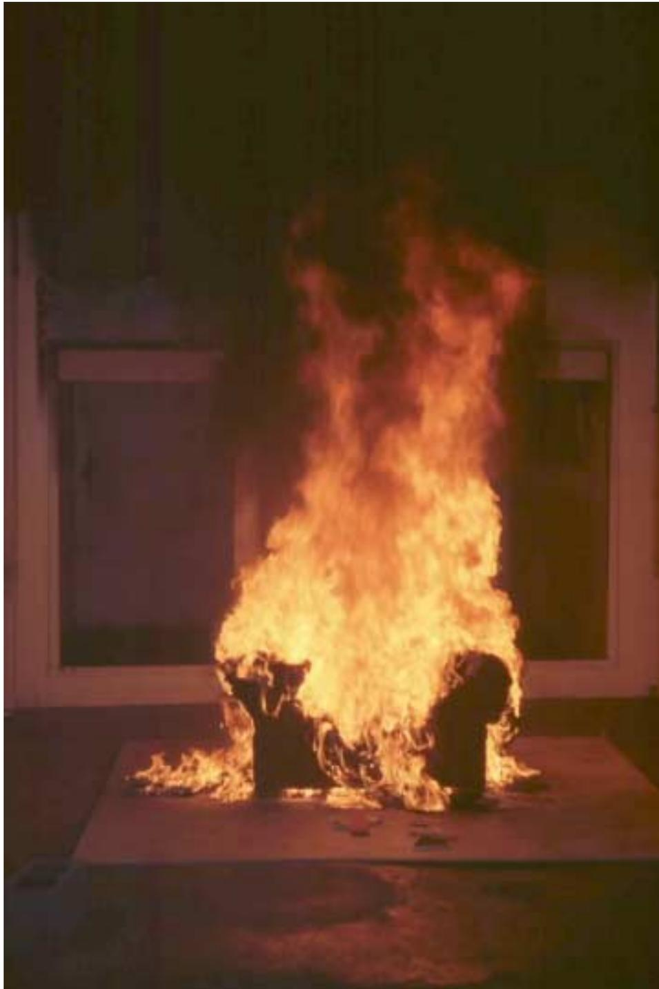
Figure 9. Photograph of chair at peak heat release rate with majority of chair burning during second test.
