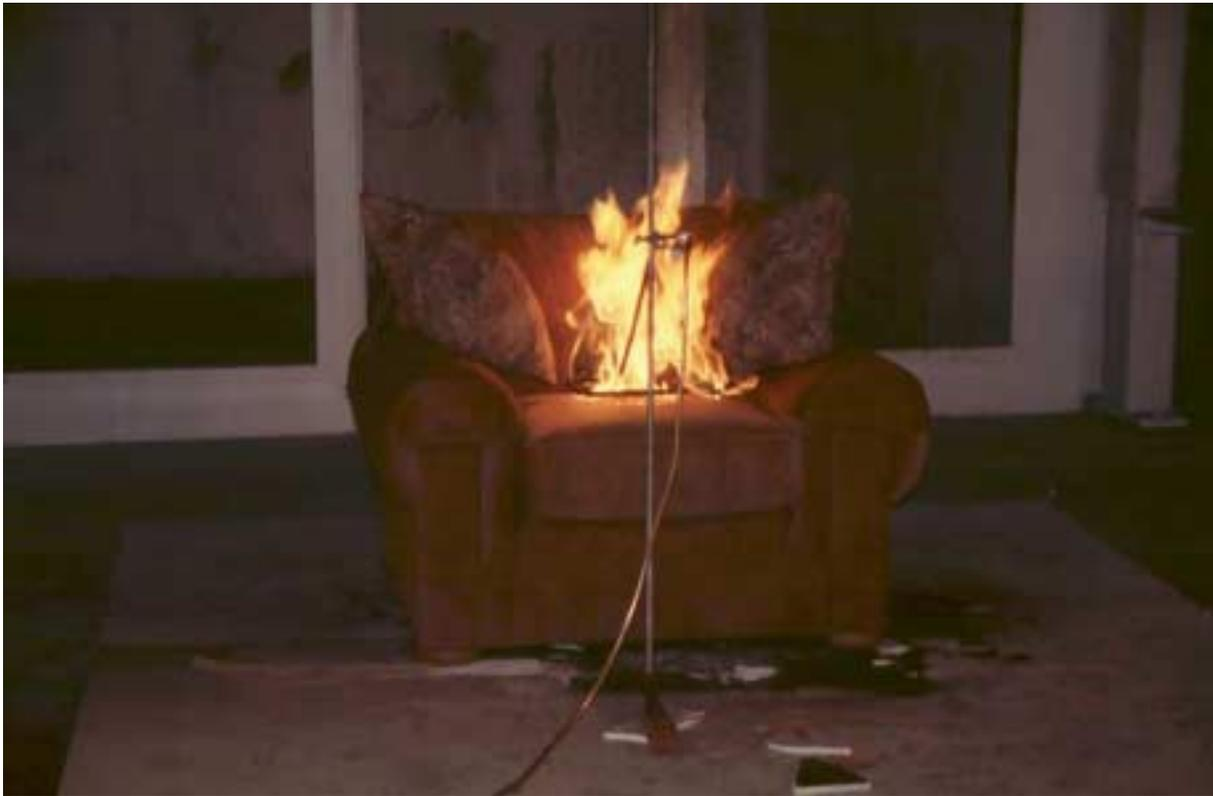
Figure 8. Photograph of chair at start of second test with CA 133 burner in place and ignited.
