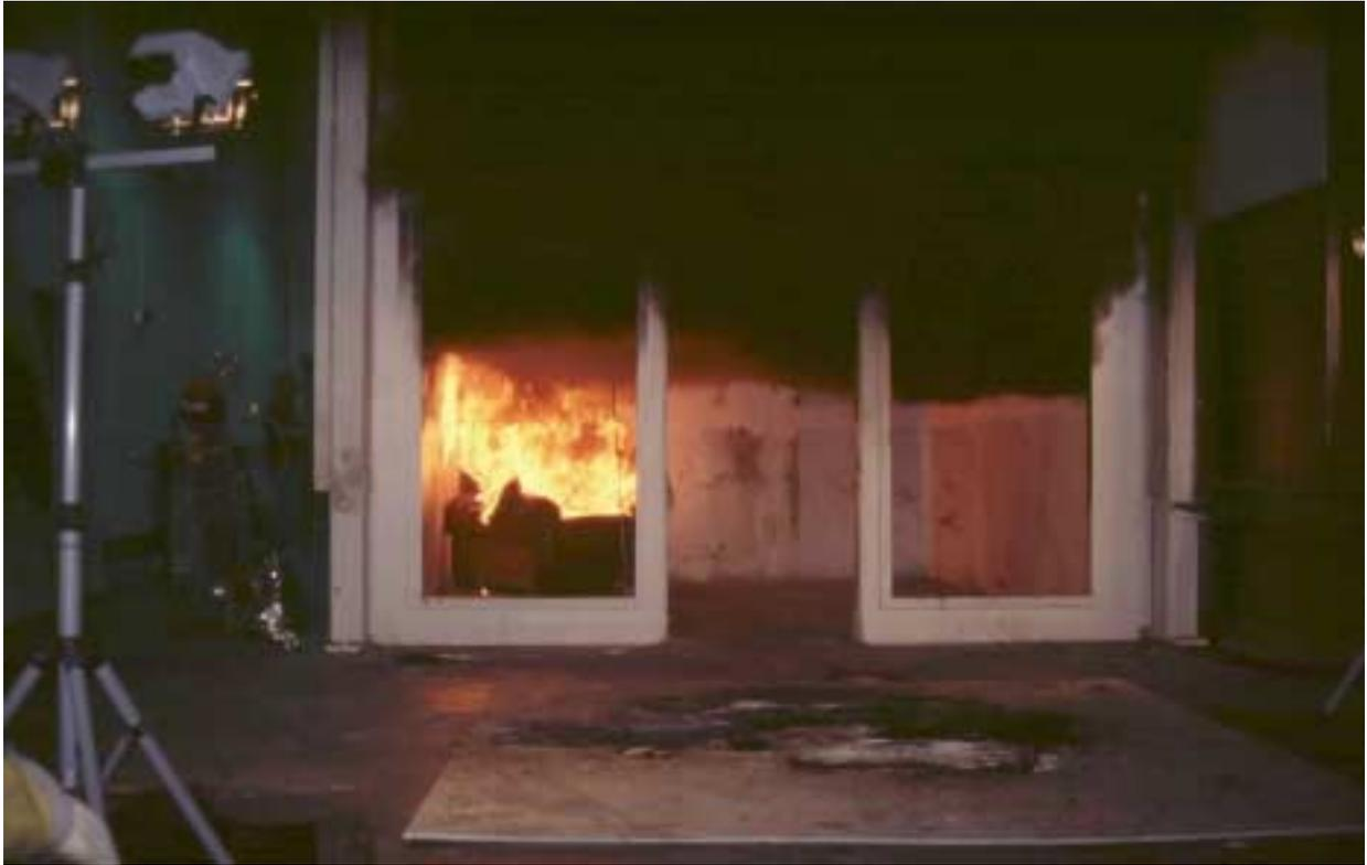
Figure 12. Photograph showing chair burning in test enclosure during the third test.
