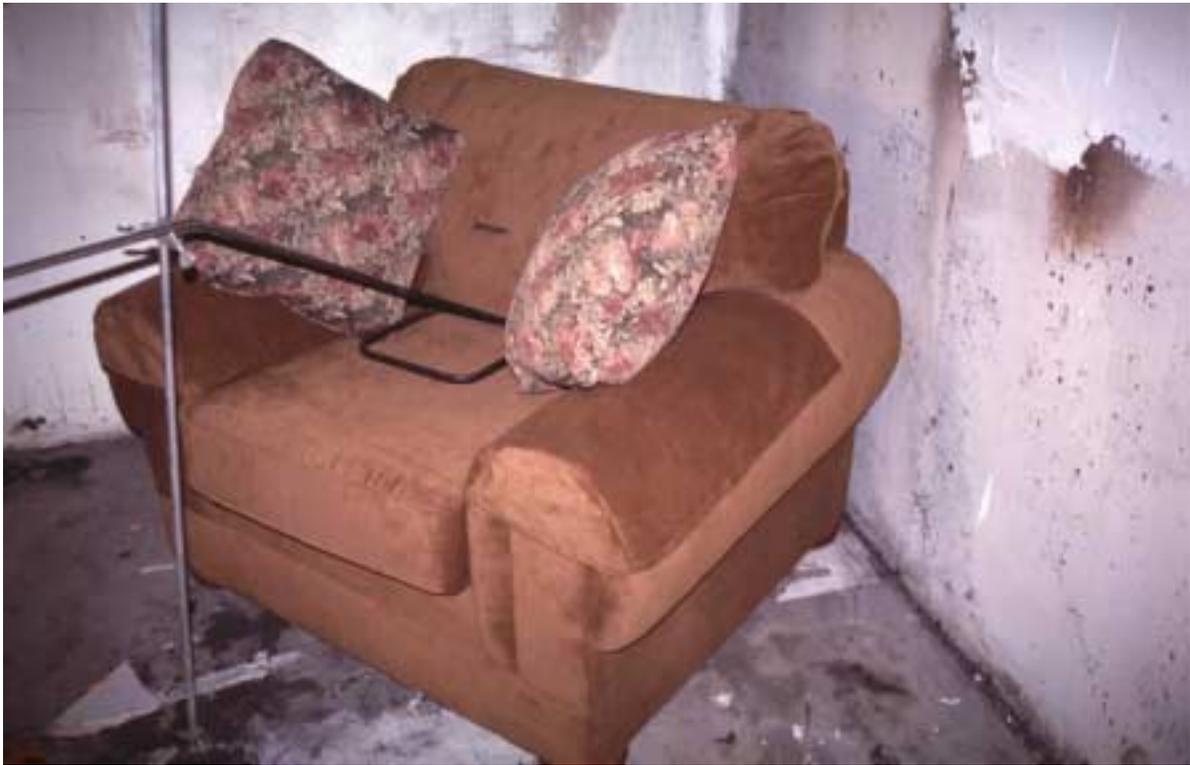
Figure 11. Photograph showing chair positioned in test enclosure with CA 133 burner in place for the third test.
