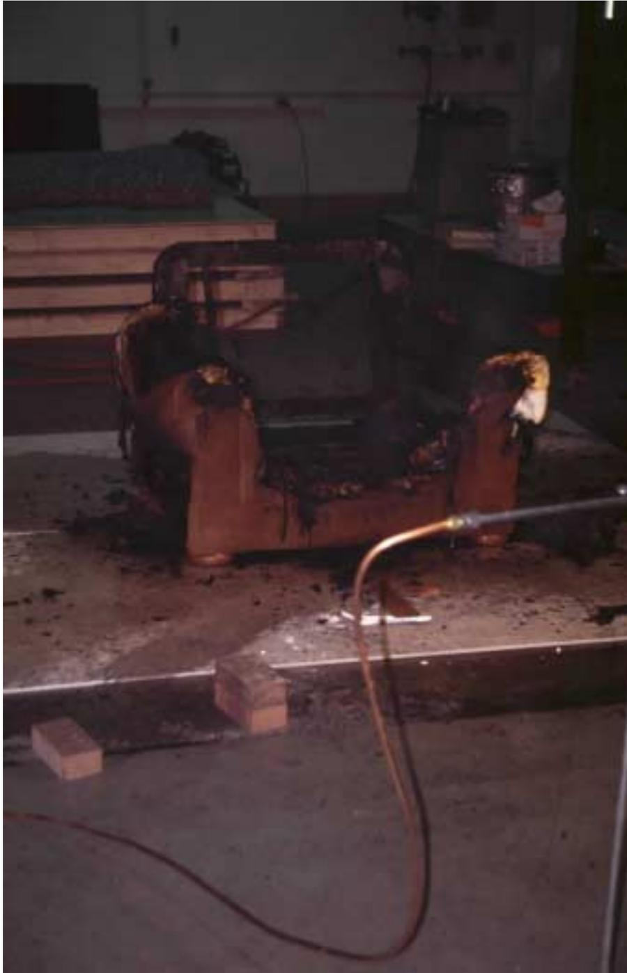
Figure 7. Photograph of chair at the end of the first test.
