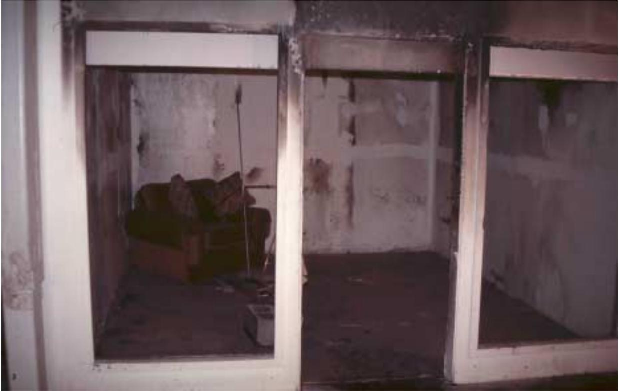
Figure 4. Photograph of a chair with CA 133 burner in placed located in a corner of a 3.7 m by 3 m by 2.4 m high test room enclosure.
