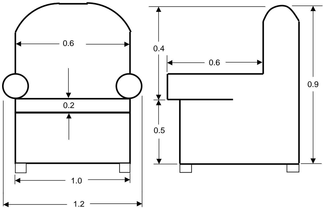
Figure 2. Front and side views of test chair with dimensions in meters.
