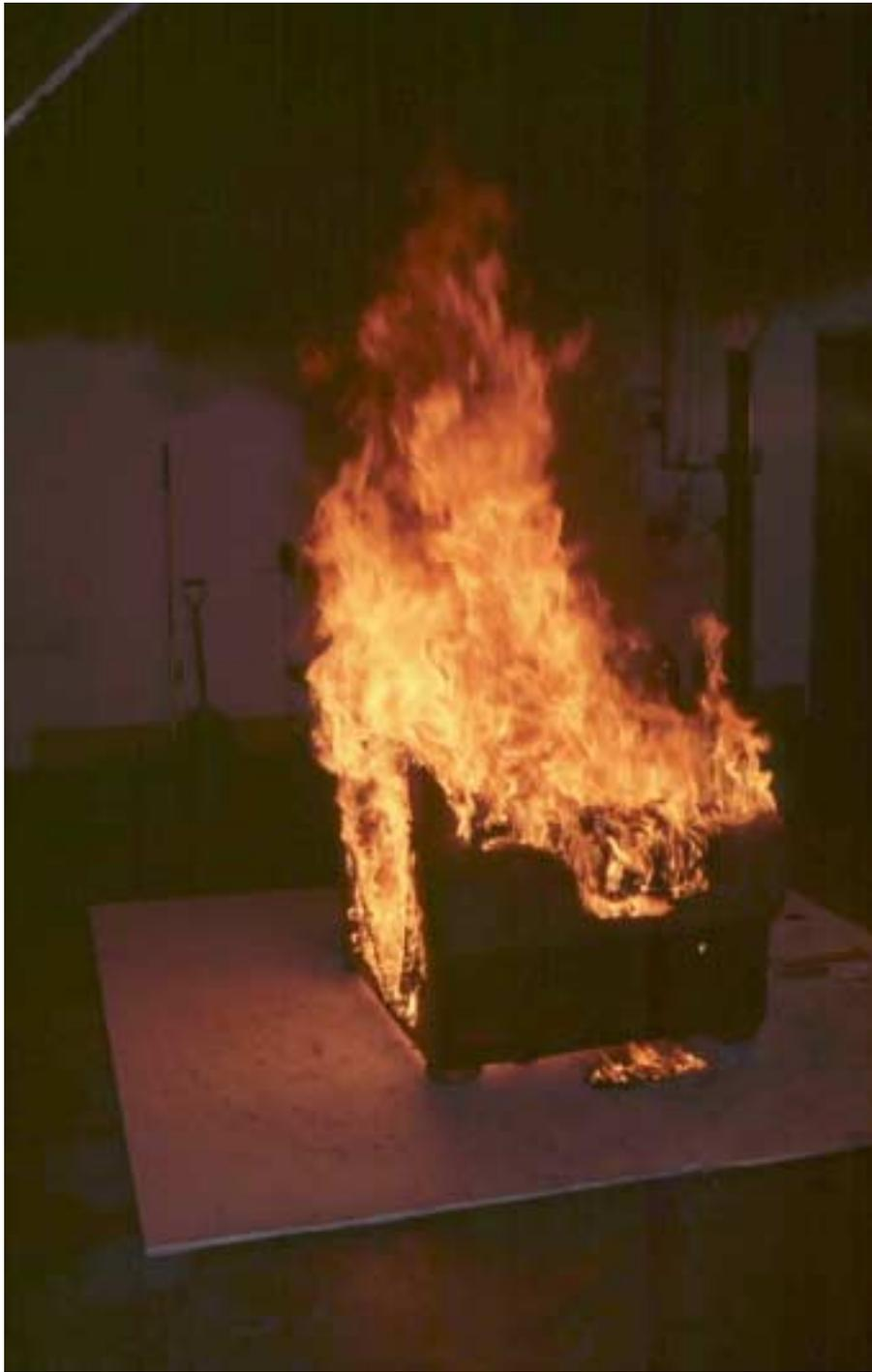
Figure 6. Photograph of chair at peak heat release rate with majority of chair burning during first test.
