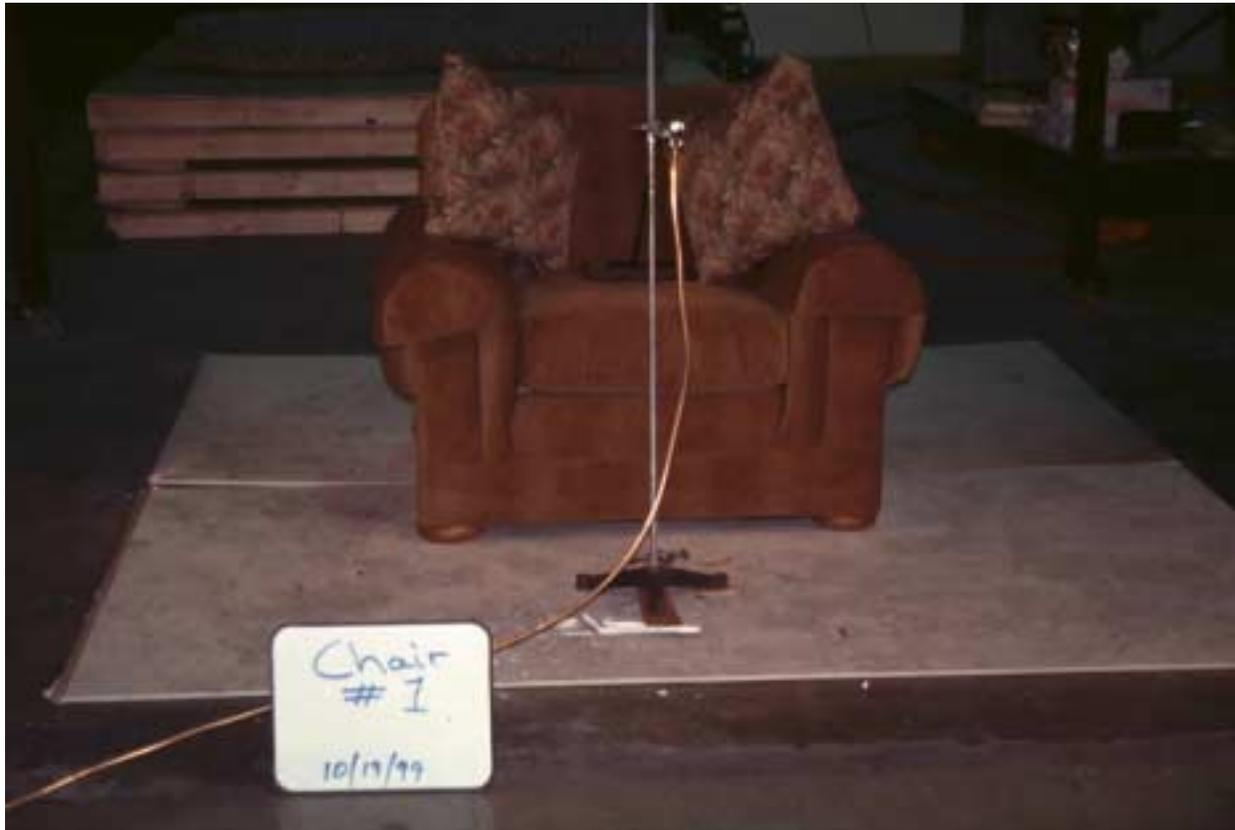
Figure 1. Photograph of chair with burner in place for start of test.
