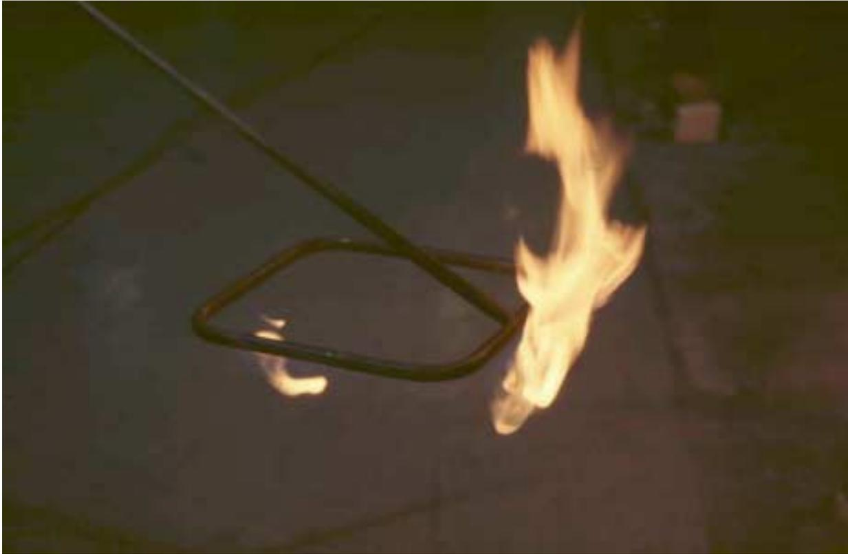
Figure 3. Photograph of CA 133 burner prior to placement on test chair.
