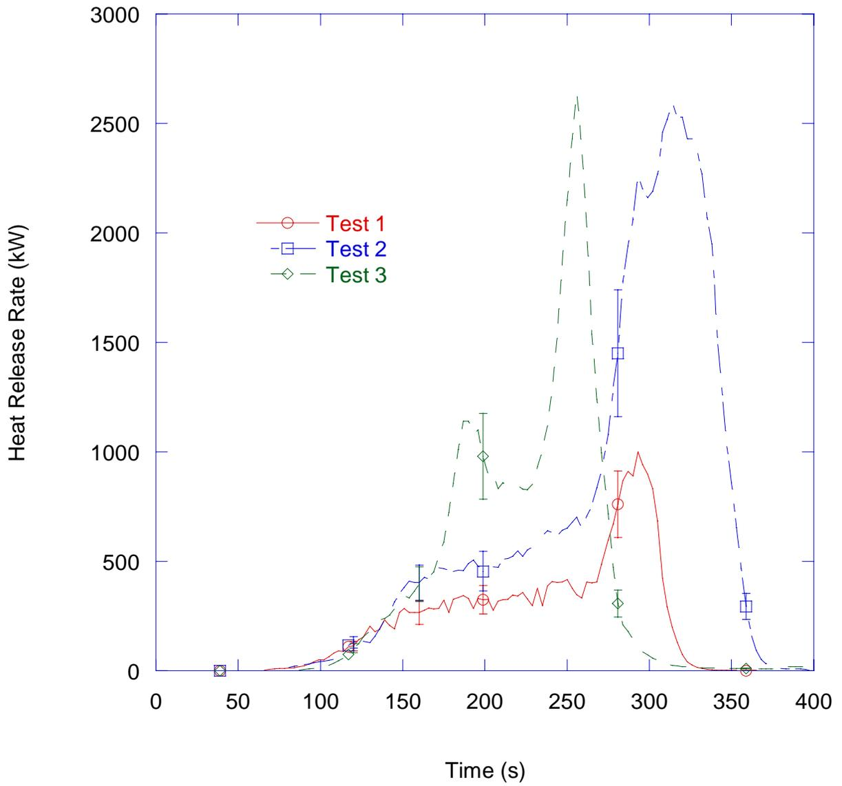
Figure 15. Graph showing heat release rate as a function of time for the three chair tests (Note: Test No. 1 exceeded the capabilities of the 500 kW hood).
