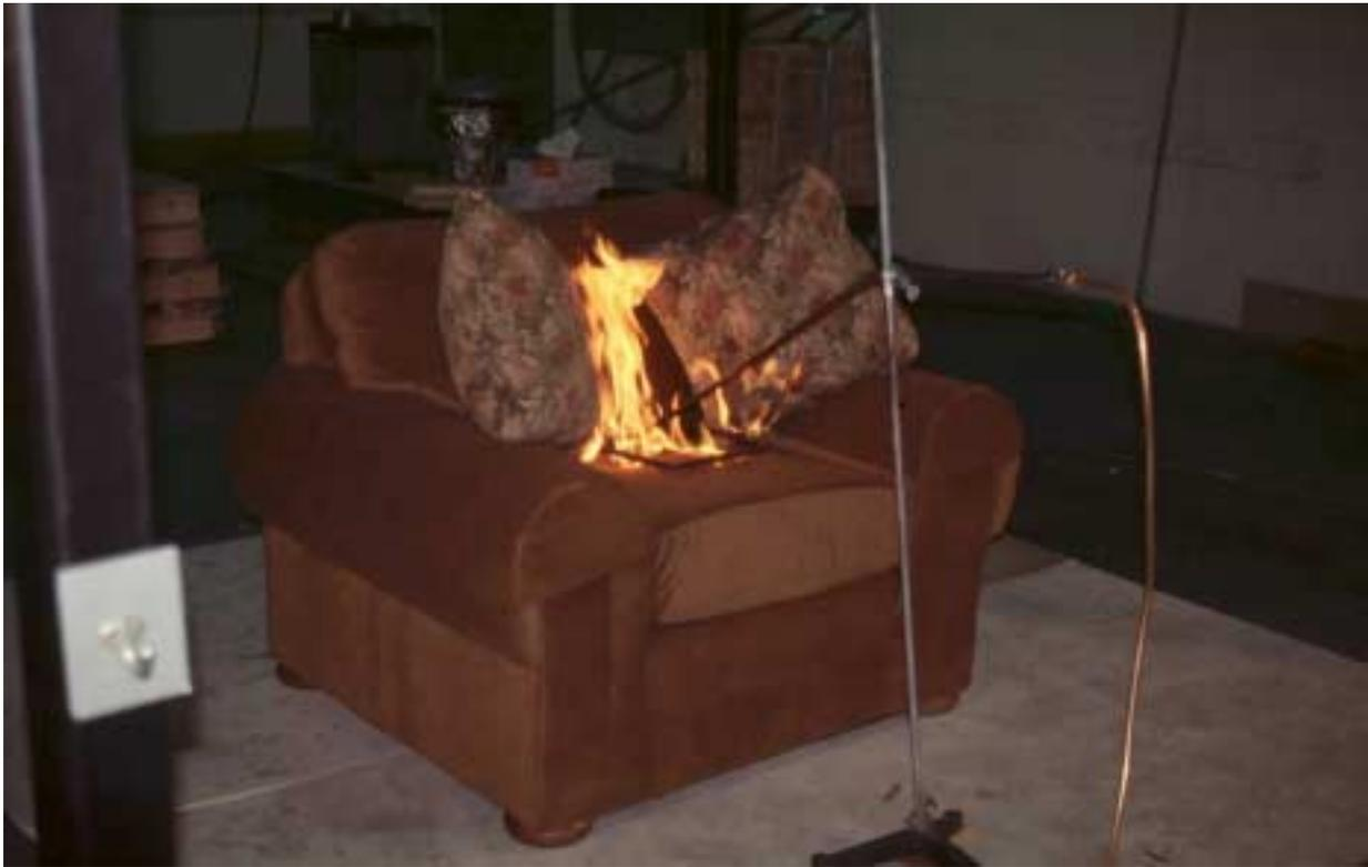
Figure 5. Photograph of chair at start of first test with CA 133 burner in place and ignited.
