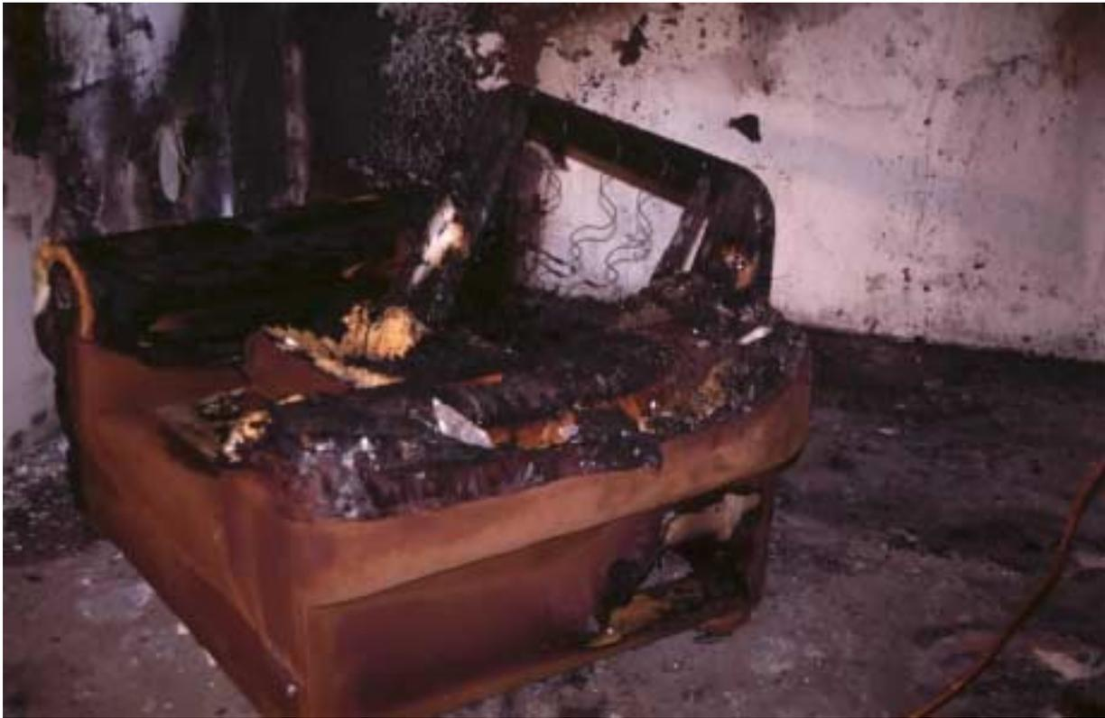
Figure 14. Photograph showing the remains of the chair and a portion of the damaged room at the conclusion of the third test.
