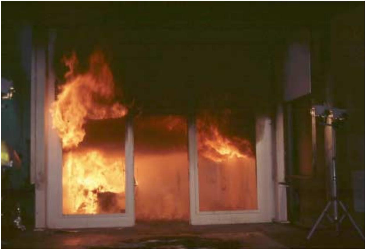
Figure 13. Photograph showing chair fully involved with fire and flames extending from the test enclosure during the third test.
