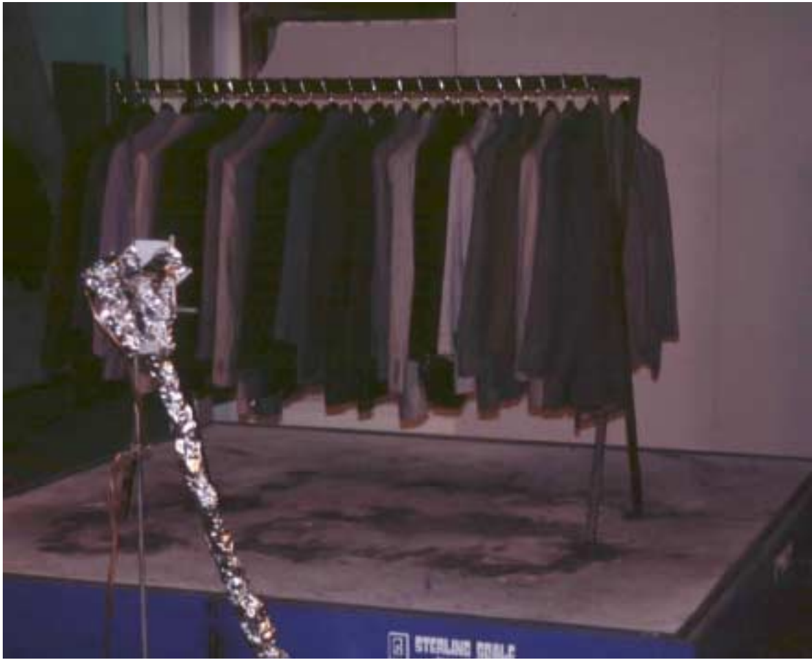
Figure 1. Photograph showing arrangement of suits on load cell.
