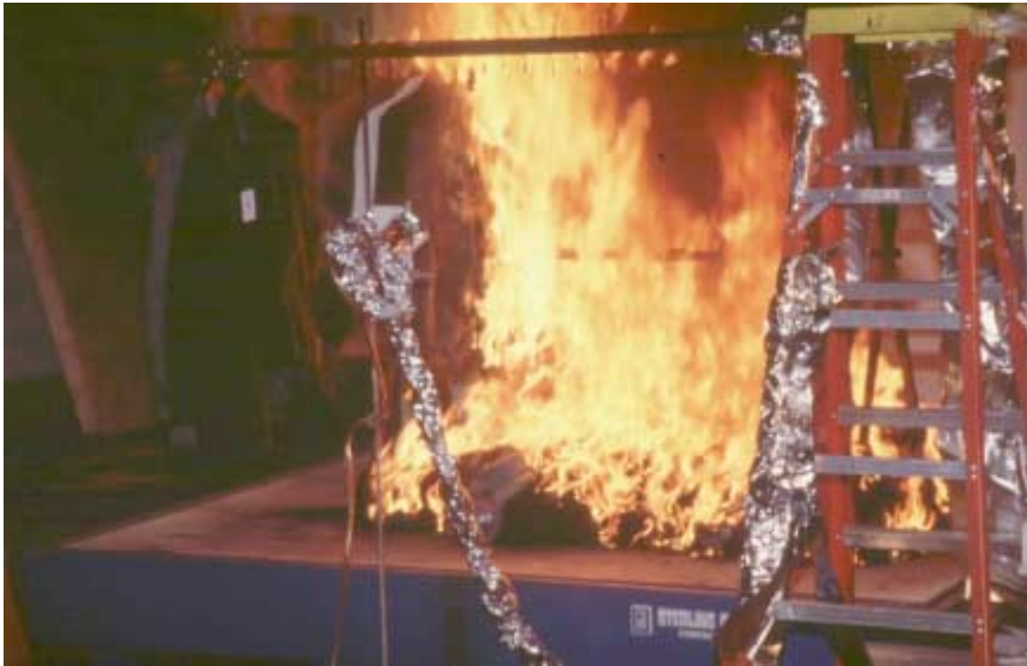
Figure 16. Photograph showing majority of suits burning during third test.
