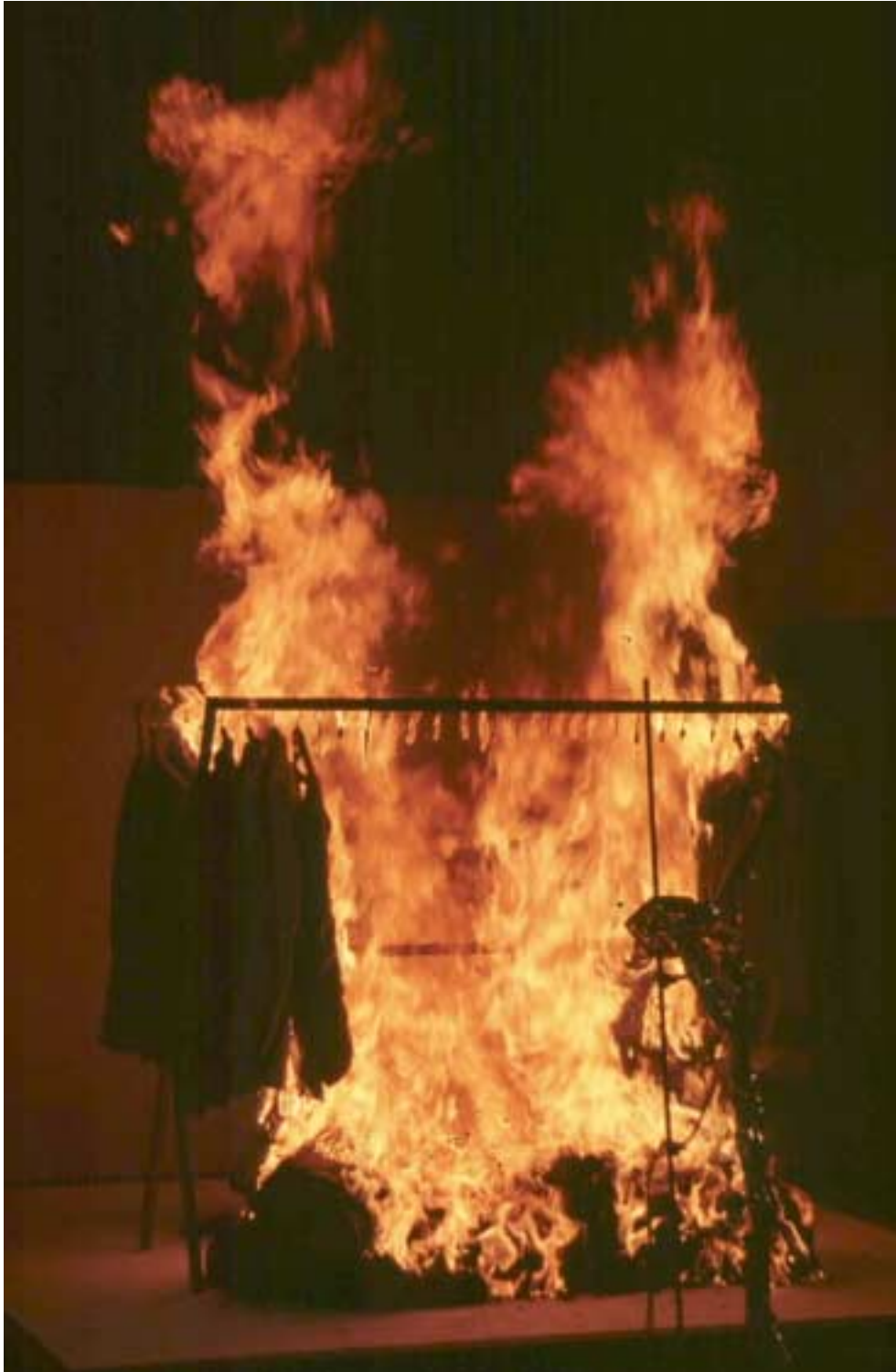
Figure 5. Photograph showing majority of suits burning during first test.
