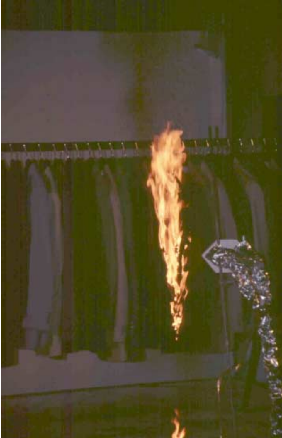
Figure 9. Photograph of suits immediately after ignition of the front, center suit for the second test.
