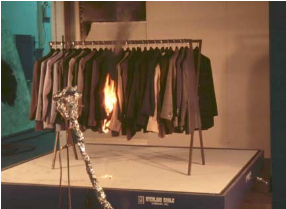
Figure 4. Photograph of suits immediately after ignition of the front, center suit for the first test.
