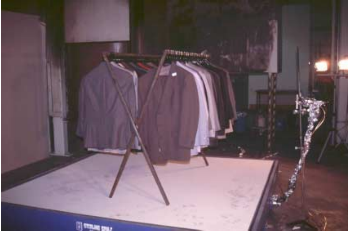
Figure 2. Photograph showing end of suit arrangement with radiometer (wrapped in aluminum foil) visible on right side.
