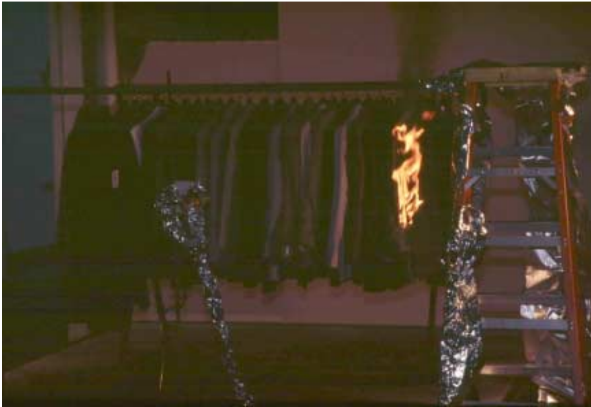
Figure 15. Photograph of suits showing fire spread along sleeve of first suit ignited during the third test.
