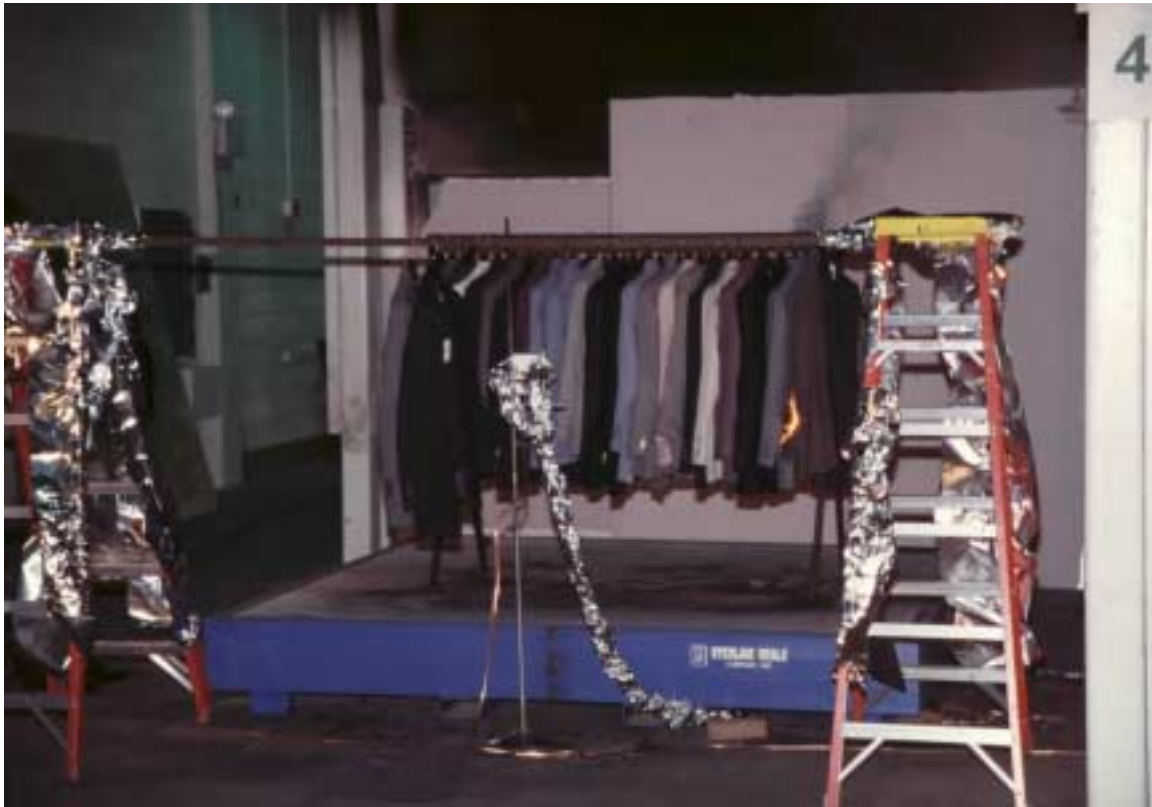
Figure 14. Photograph of suits immediately after ignition of the front, right end suit for the third test.
