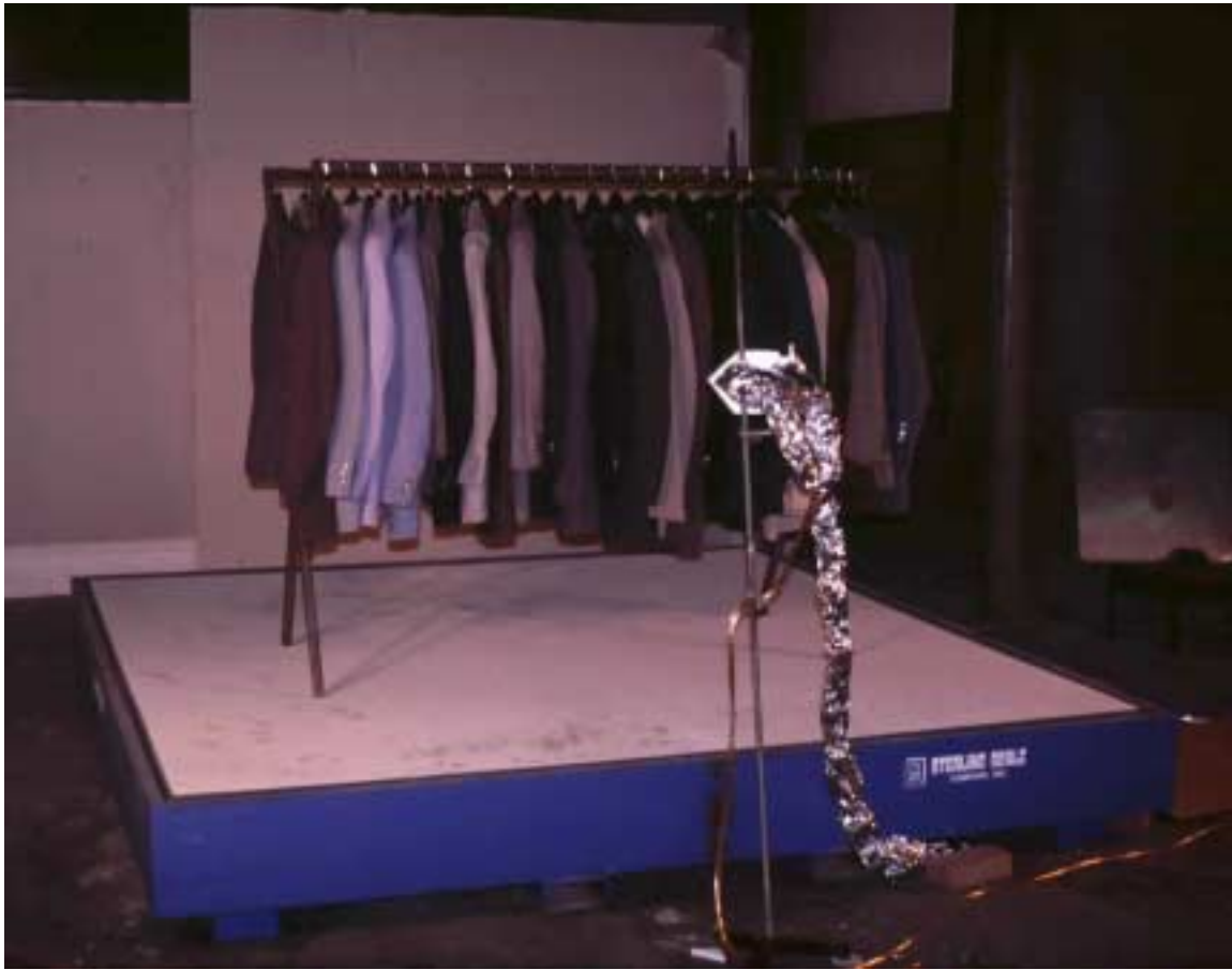
Figure 8. Photograph of suit arrangement for the second test.
