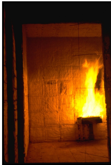
Figure 2-3: Photo of a 100 kW fire with the burner located against the rear wall of one of the small compartments. Photo provided by Rick Peacock, NIST.
