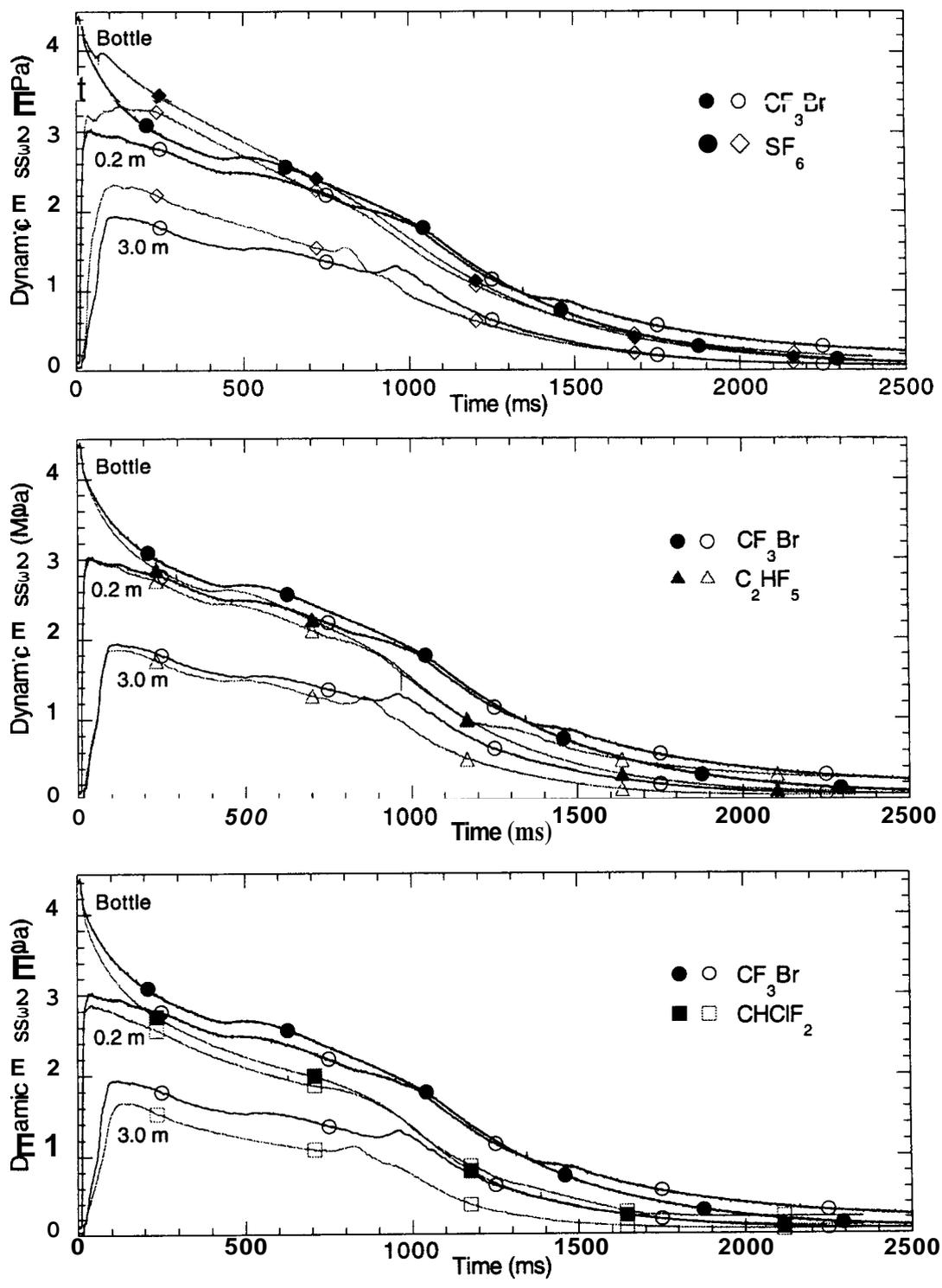
Figure 3: Pressure traces in the vessel (solid markers) and located 0.2 m and 3.0 m downstream (outline markers) of NIST discharges to atmosphere: (a) SF<sub>6</sub> and CF<sub>3</sub>Br, (b) C<sub>2</sub>HF<sub>5</sub> and CF<sub>3</sub>Br, and (c) CHClF<sub>2</sub> and CF<sub>3</sub>Br.
