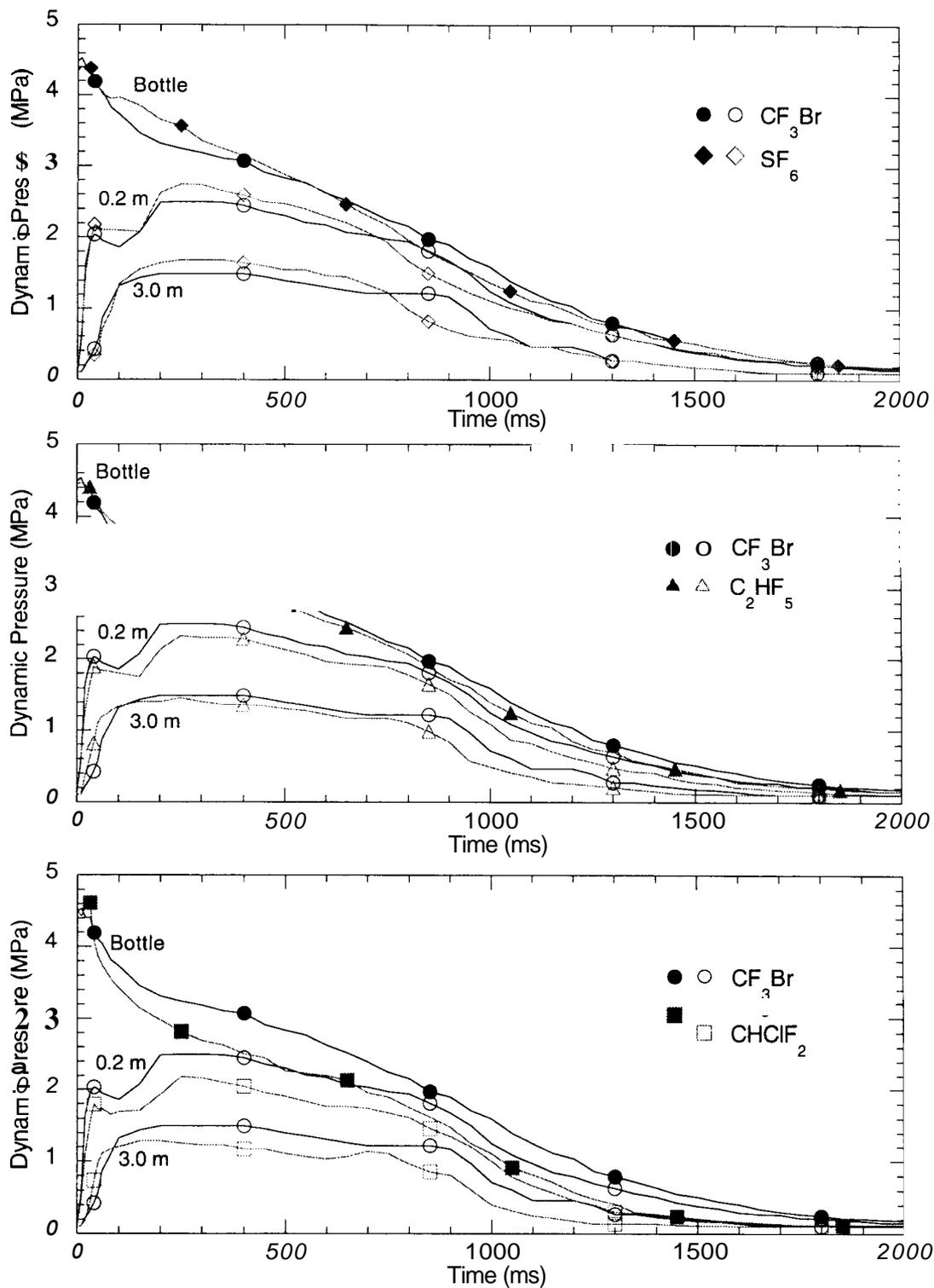
Figure 2: Pressure traces in the vessel (solid markers) and located 0.2 m and 3.0 m downstream (outline markers) of WKA discharges to atmosphere: (a)  $\text{SF}_6$  and  $\text{CF}_3\text{Br}$  and (b)  $\text{C}_2\text{HF}_5$  and  $\text{CF}_3\text{Br}$ ; and into a 900 liter recovery tank: (c)  $\text{CHClF}_2$  and  $\text{CF}_3\text{Br}$ .
