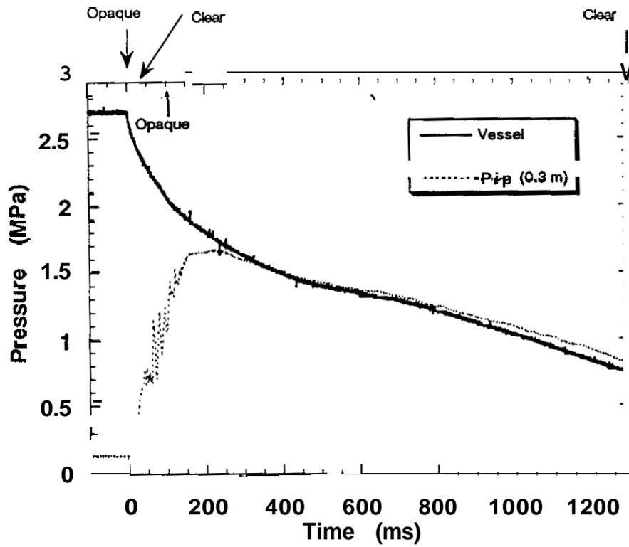
Figure 4. Pressure traces for HFC-227ea tested at a 50% fill condition, pressurized to 2.8 MPa with no make-up nitrogen addition. Arrows indicate the approximate time of the high speed movie observation.
