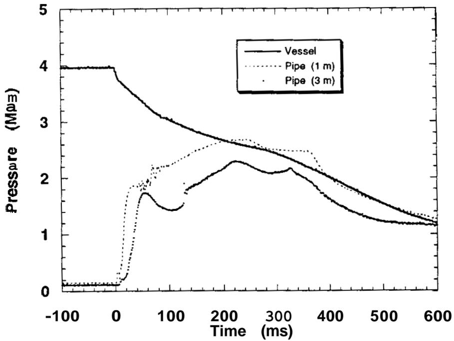
Figure 7. Pressure traces for halon 1301 tested at a 50% fill condition, pressurized to 4.1 MPa with no make-up nitrogen addition.
