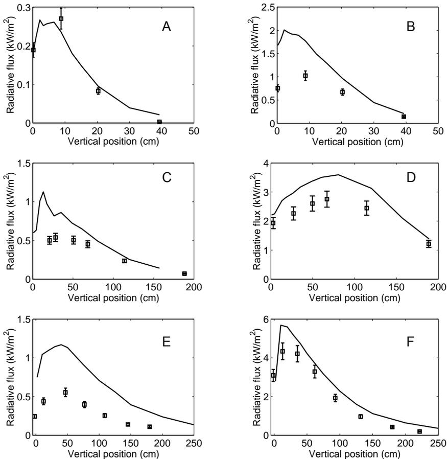
Fig. 3. - Comparison of the measured (squares) and predicted (lines) vertical heat flux distributions outside the methane flames.
