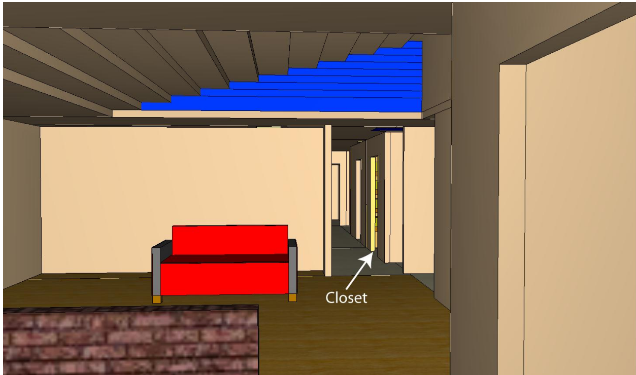
Figure 14: View of the simulated gypsum failure area (blue) from behind the brick knee wall in the kitchen.
