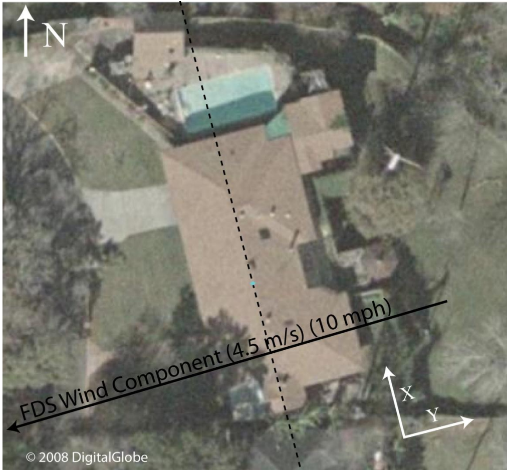
Figure 18: Wind vector orthogonal to the computational domain. Background image used with permission of Digital Globe. Enhancements by NIST.
