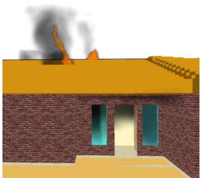
Figure 29: Roof one minute after vent is opened, when first fire is seen in no-wind simulation
