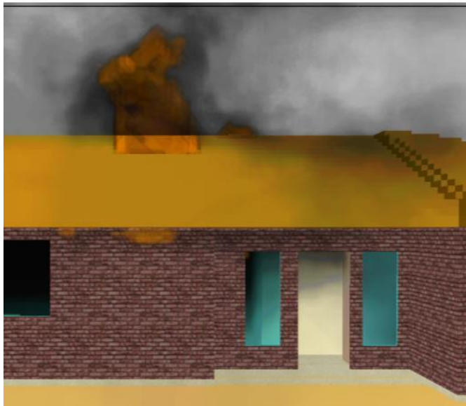
Figure 28: Roof immediately after vent is opened in wind simulation
