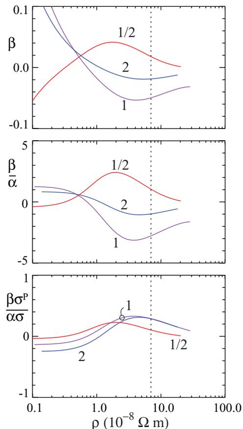
FIG. 5. (Color online) Spin-transfer torque parameter versus resistivity for several ratios ( $r = 0.5, 1.0, 2.0$ ) of spin-dependent scattering rates for Ni. The top panel gives  $\beta$ , the middle panel  $\beta/\alpha$ , and the bottom panel  $\beta\sigma_P/(\alpha\sigma)$ . The dashed vertical lines indicate the approximate room-temperature resistivity.
