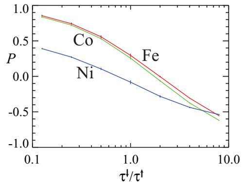
FIG. 2. (Color online) Polarization for bcc Fe (red), hcp Co (green), fcc Ni (blue) as a function of the ratio of lifetimes for the two spin channels,  $r = \tau^\downarrow/\tau^\uparrow$ . At each value of  $r$ ,  $P$  is calculated for a range of  $\tau^\uparrow$  and  $\tau^\downarrow$  and the range of resulting values is indicated by the vertical bar at each data point.
