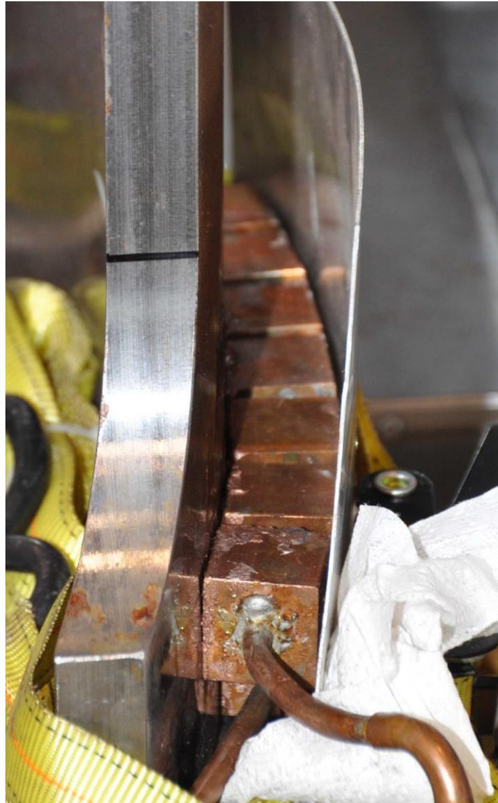
Figure 22. Bottom cooling blocks installed on a CWP specimen.
