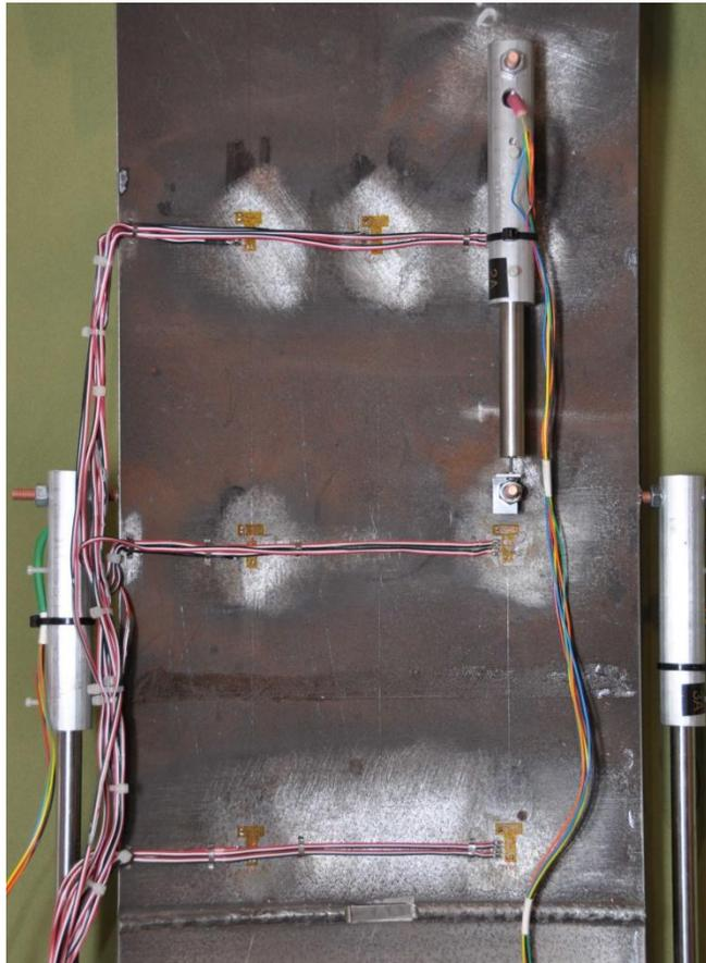
**Figure 6. Photograph of the ID surface of a specimen, showing the minimal surface changes necessary to prepare the surface for instrumentation. Strain gages and LVDTs are installed on the specimen in this photo. This was a room-temperature test, so thermocouples are absent; however, the area necessary to install thermocouples was very small.**
