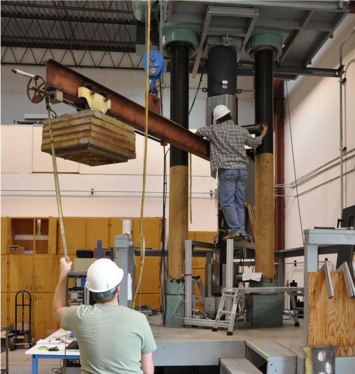
**Figure 23. Photograph taken during the specimen installation process. The movable counter-balance strong-back was supported by the overhead crane, allowing adequate reach into the test frame, where the overhead crane had no direct access, because of the crosshead.**
