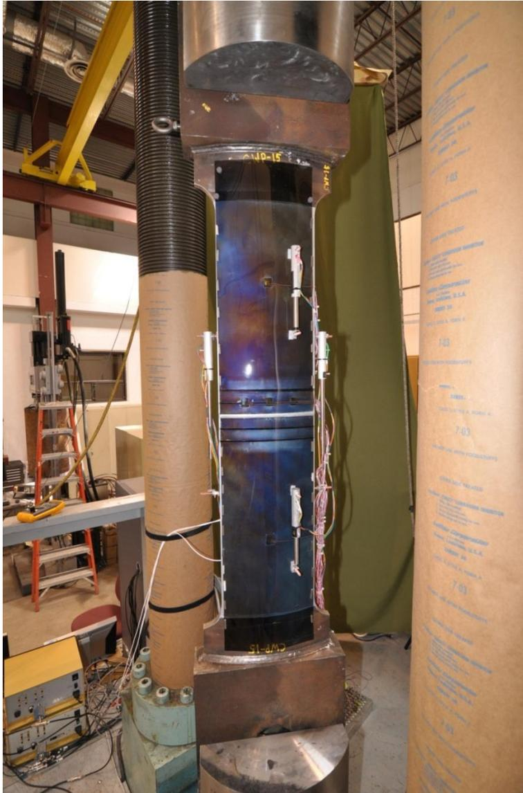
**Figure 16. Outside diameter side of the specimen showing the installation of the photoelastic film covered by the polarizing sheets on the specimen. Cut-outs in the photoelastic and polarizing film allowed the installation of the LVDTs and strain gages.**
