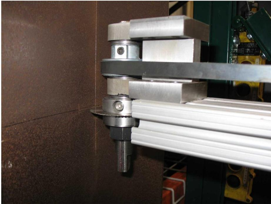
**Figure 7. Photograph of the slitting saw head close to the ID surface of the base metal specimen**
