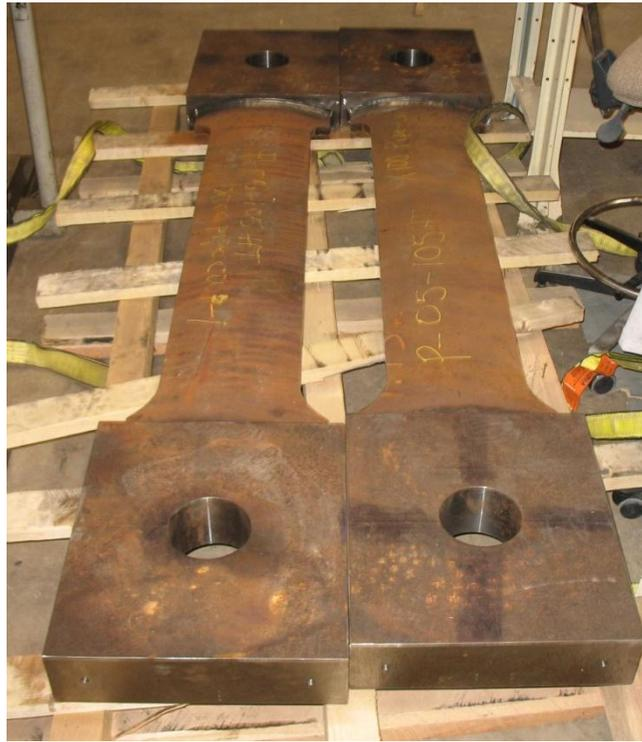
**Figure 4. First shipment of specimens received at NIST. The first two specimens were base metal specimens without girth welds.**
