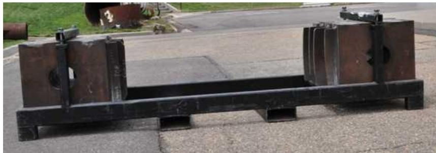
**Figure 5. Shipping crate designed and fabricated at Lincoln Electric for shipping CWP specimens between NIST and Lincoln Electric.**
