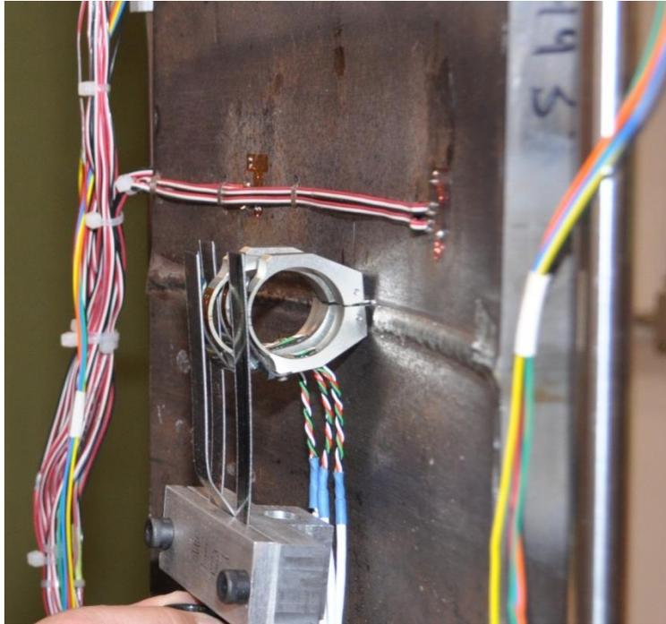
Figure 18. Inside-diameter side of the specimen, showing the installation of the CMOD gauges in the notch.
