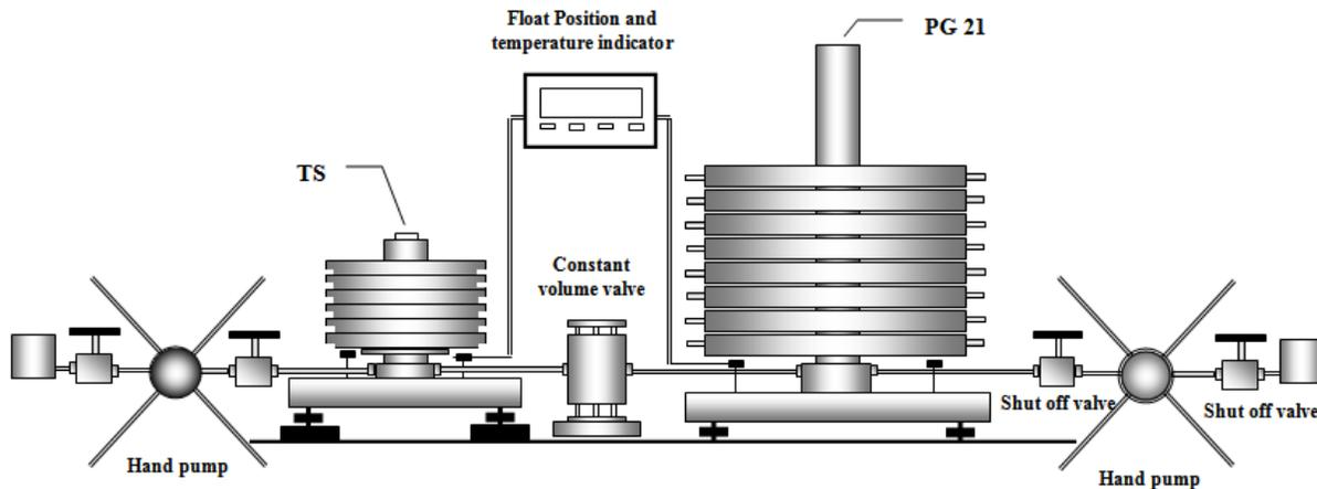
Fig.2.NIST experimental set-up showing the crossfloat system of TS versus LS.
