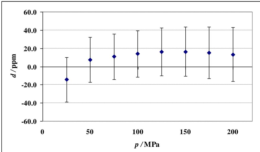
Fig. 4. Degree of equivalence between NIST and NIS plotted as the relative difference in effective area vs. pressure. Error bars are the standard uncertainty of the difference.
