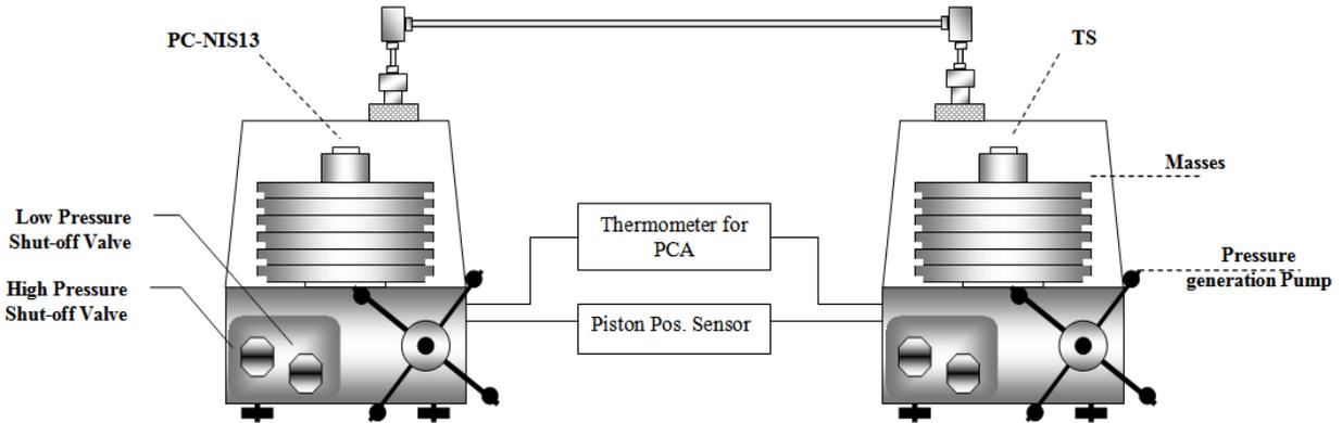
Fig. 3. NIS experimental set-up shows the crossfloat system of TS versus LS.
