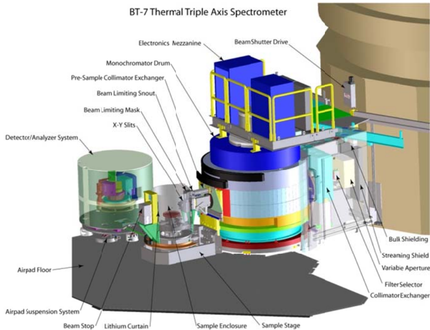
Figure 1. Cut-away layout of the new instrument. The size of the beam exiting from the source can be varied by a set of x - y slits, and can pass through a filter and a system with a selection of horizontal collimations, before striking the double-focusing monochromator. The monochromatic beam impinges on the sample table that is cantilevered from the monochromator drum. The analyzer system is on air pads.
