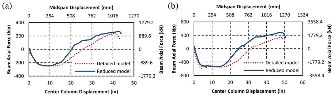
Fig. 6. Beam axial forces versus vertical displacement of center stub column for (a) IMF specimen and (b) SMF specimen
