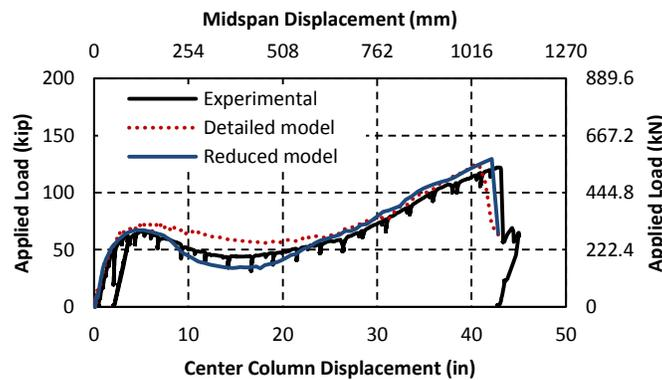
Fig. 4. Vertical load versus vertical displacement of center stub column for the IMF specimen
