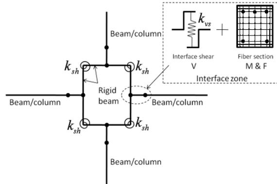
Fig. 1. Reduced beam-to-column connection model
