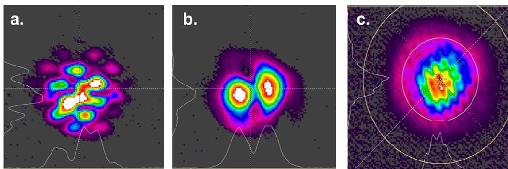
**Fig. 7.** These images depict the various states of seed beam alignment a. grossly misaligned, b. aligned to higher order modes, c. aligned and locked to the cavity. The distortion observed in c. is due to interference on the output coupler
