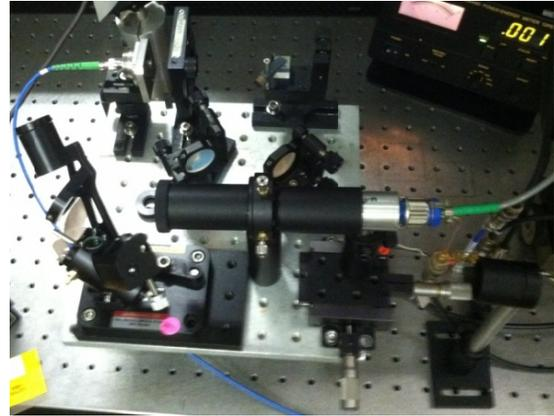
**Fig. 3.** Mounted to a 9" x 9" breadboard are the fiber output from the seed laser, polarizing beam splitter cube, seed alignment mirrors, RISTRA cavity (lower left in picture), and the fringe detector. Long pass filters (LPF), (OD 6 at 1064 nm) are used to attenuate the residual pump pulse. Mirrors 1- 4 are labeled.
