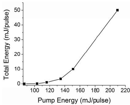
**Fig. 8.** Efficiency curve using two critically phase matched KTA crystals and with seeded input. The seed laser was locked to a mode of the RISTRA cavity for all measurements.
