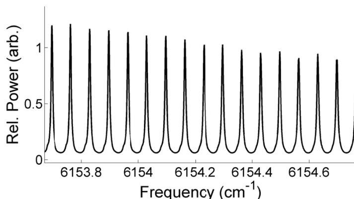
**Fig. 6** Measured longitudinal mode structure of RISTRA cavity. The data was acquired by scanning the diode laser through the fringes of the cavity while recording the output power on the fringe detector and the frequency of the diode laser.
