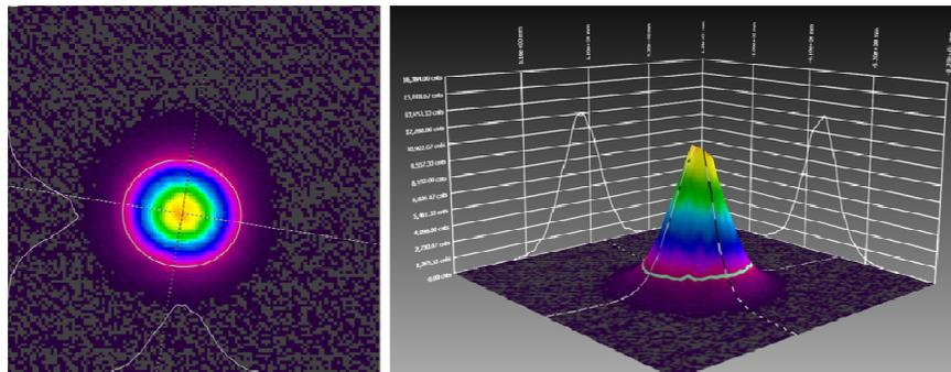
**Fig. 4.** Seed beam spatial fluence profile is shown as a contour and surface plots
