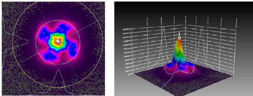
**Fig. 9** The RISTRA OPO output spatial fluence profile is shown as a contour and surface plots. We believe that an improvement in our pump laser mode quality will result in improved mode quality from the OPO.
