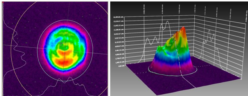
**Fig. 2** The pump laser spatial fluence profile is shown as a contour and surface plots.
