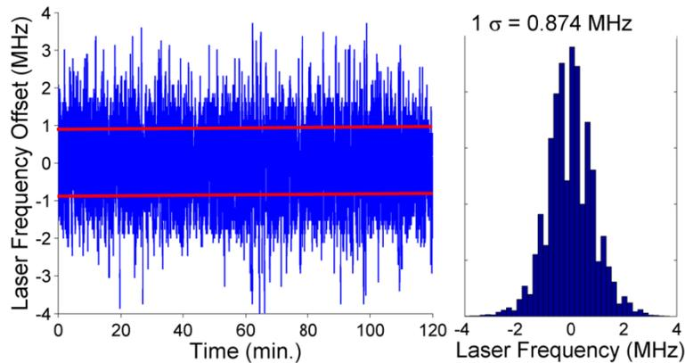
**Fig. 5.** Long term wavelength stability showing a time trace of the laser frequency and a histogram of the amount of time spent in different frequency bins over the 120 minute observation period.
