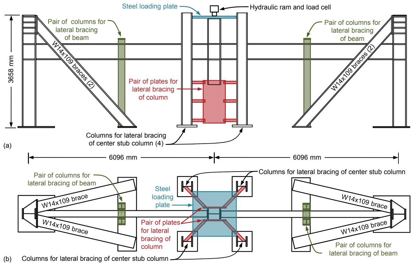
**Fig. 3.** Schematic of test setup: (a) elevation view; (b) plan view
