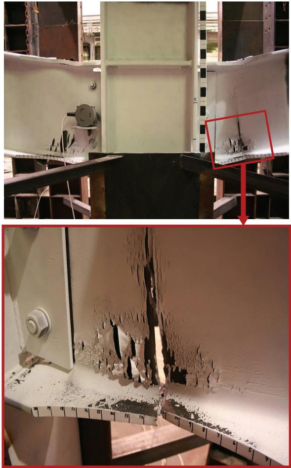
**Fig. 12.** Failure mode of RBS specimen
