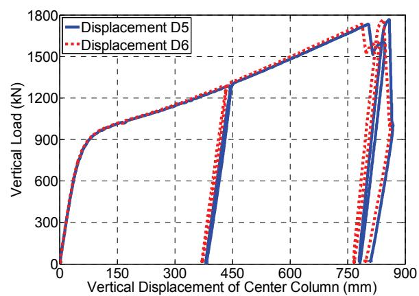
**Fig. 14.** Vertical load versus center column displacement for RBS specimen
