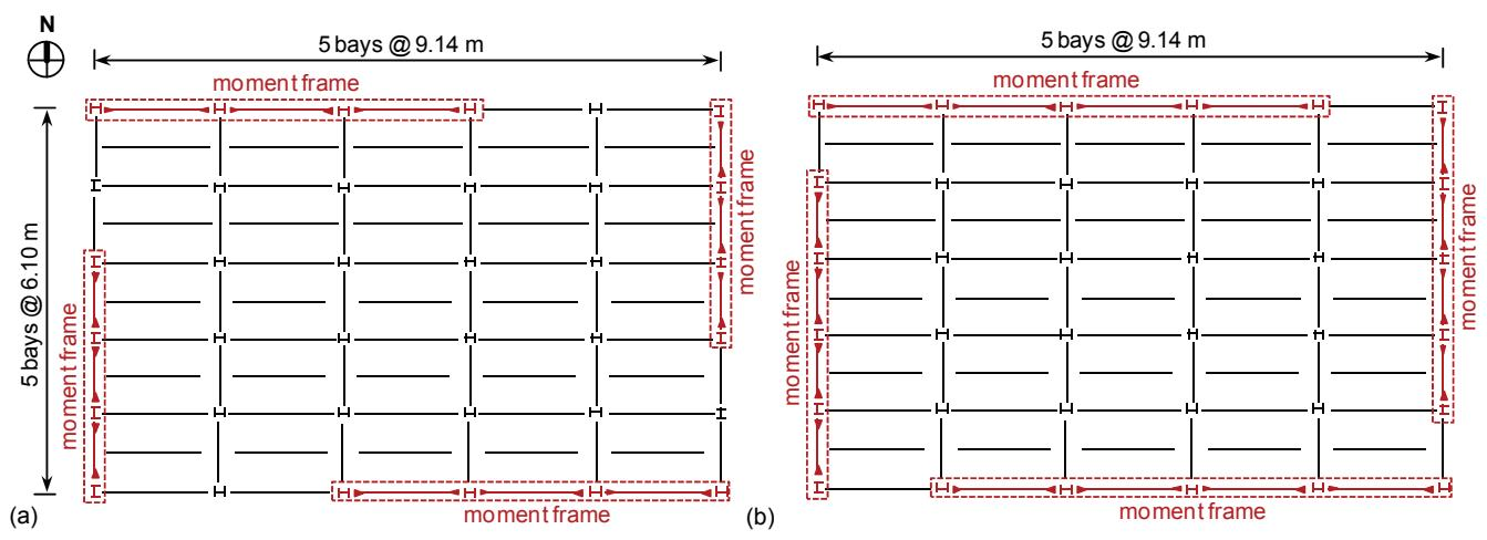
**Fig. 1.** Plan layouts for (a) SDC C building and (b) SDC D building
