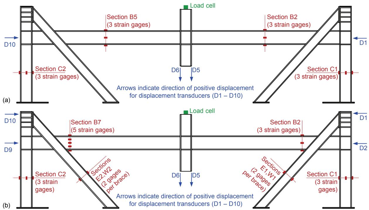
**Fig. 5.** Selected instrumentation for (a) WUF-B specimen and (b) RBS specimen
