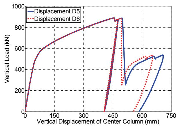
**Fig. 8.** Vertical load versus center column displacement for WUF-B specimen
