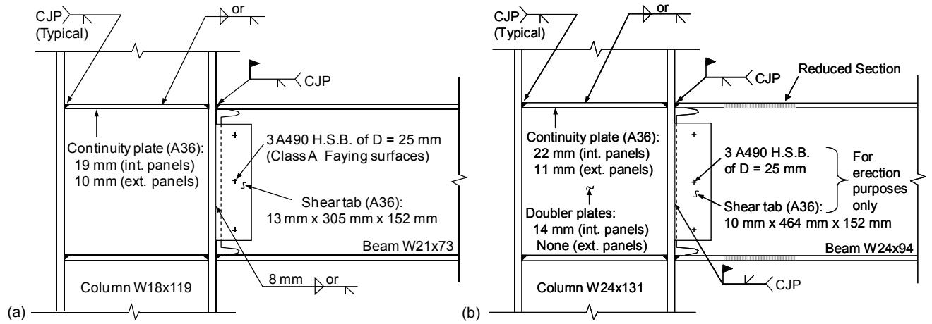
**Fig. 2.** Moment connection details: (a) WUF-B connection; (b) RBS connection
