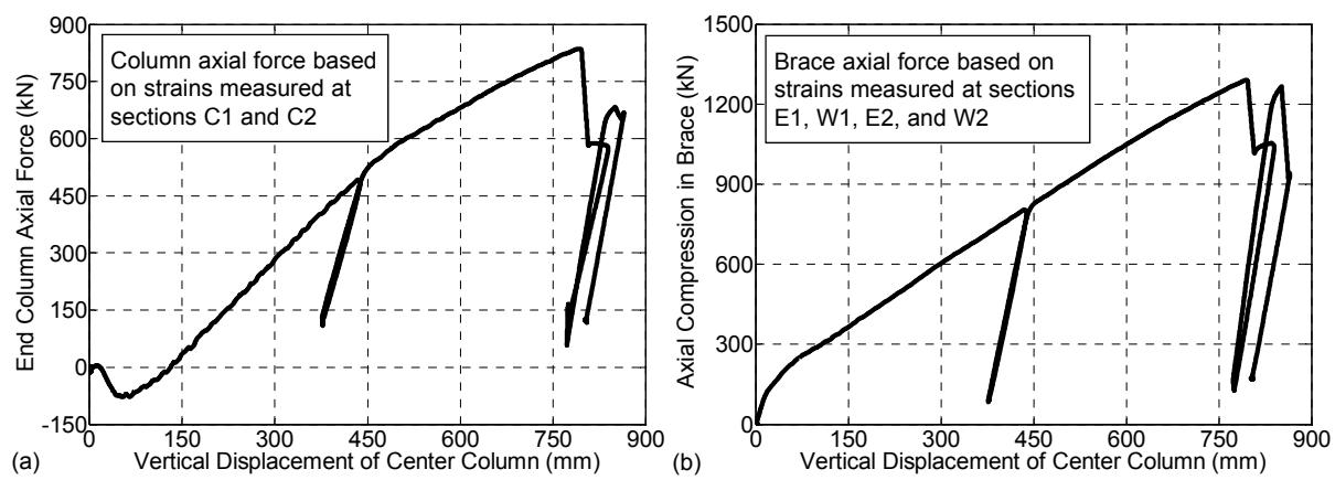
**Fig. 17.** (a) Axial force in end columns and (b) axial compression in diagonal braces versus center column displacement for RBS specimen
