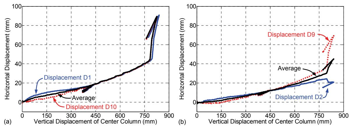
**Fig. 15.** Horizontal displacement of end columns at (a) top of columns and (b) mid-height of beams versus center column displacement for RBS specimen
