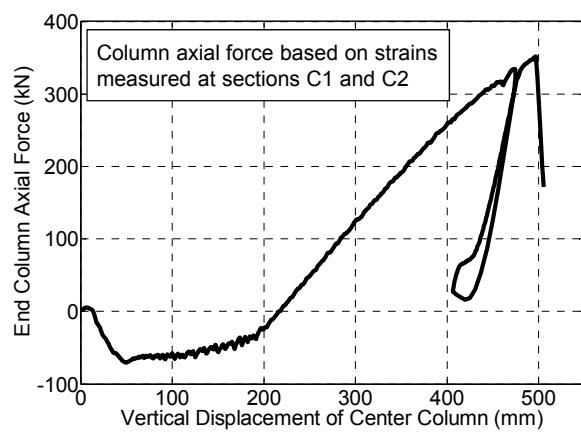
**Fig. 11.** Axial force in end columns versus center column displacement for WUF-B specimen
