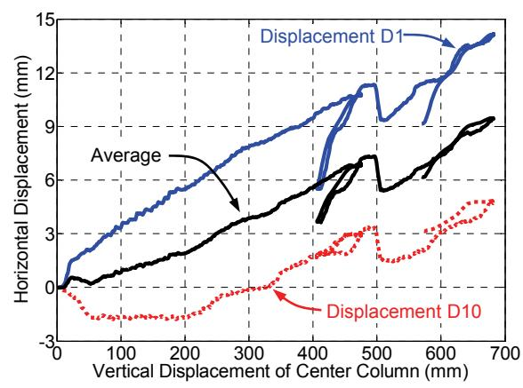
**Fig. 9.** Horizontal displacement of end columns at beam mid-height versus center column displacement for WUF-B specimen
