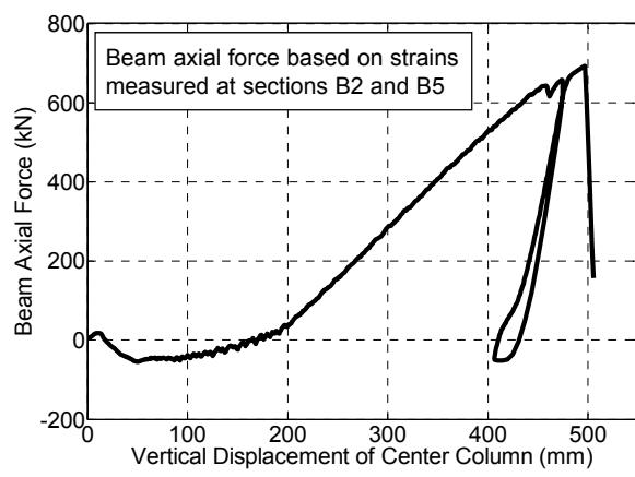
**Fig. 10.** Axial force in beams versus center column displacement for WUF-B specimen
