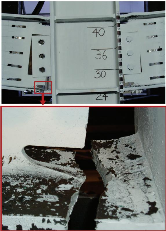
**Fig. 6.** Failure mode of WUF-B specimen
