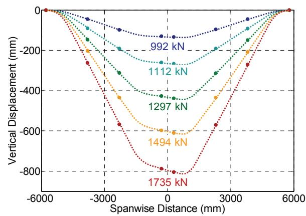
**Fig. 13.** Vertical displacement profile of beams corresponding to indicated vertical loads for RBS specimen (displacements magnified)
