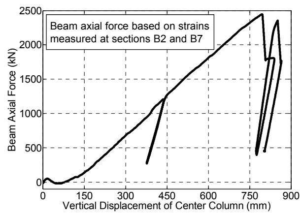
**Fig. 16.** Axial force in beams versus center column displacement for RBS specimen
