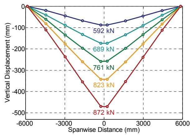
**Fig. 7.** Vertical displacement profile of beams corresponding to indicated vertical loads for WUF-B specimen (displacements magnified)
