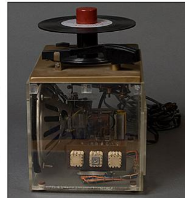
Project Tinkertoy Wafer Tube Amplifier
