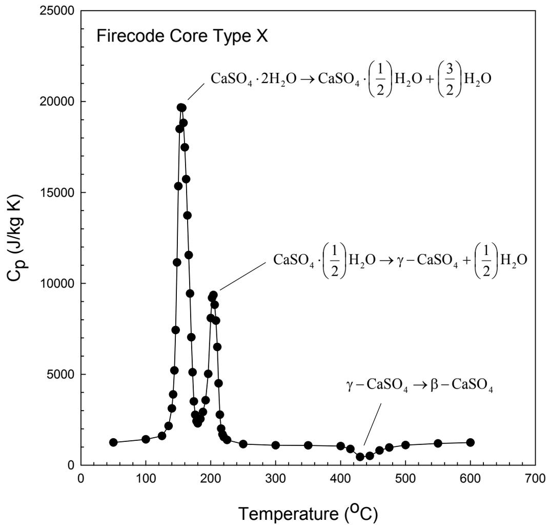
Figure B-1. Specific heat capacity of Firecode CoreType X 5/8 in. gypsum.
