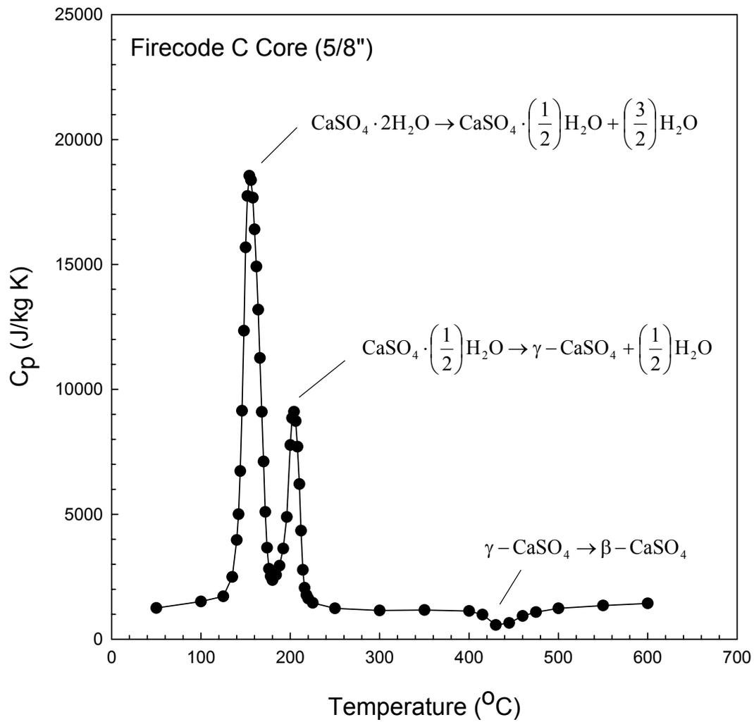
Figure B-3. Specific heat capacity of Firecode C Core 5/8 in. gypsum.
