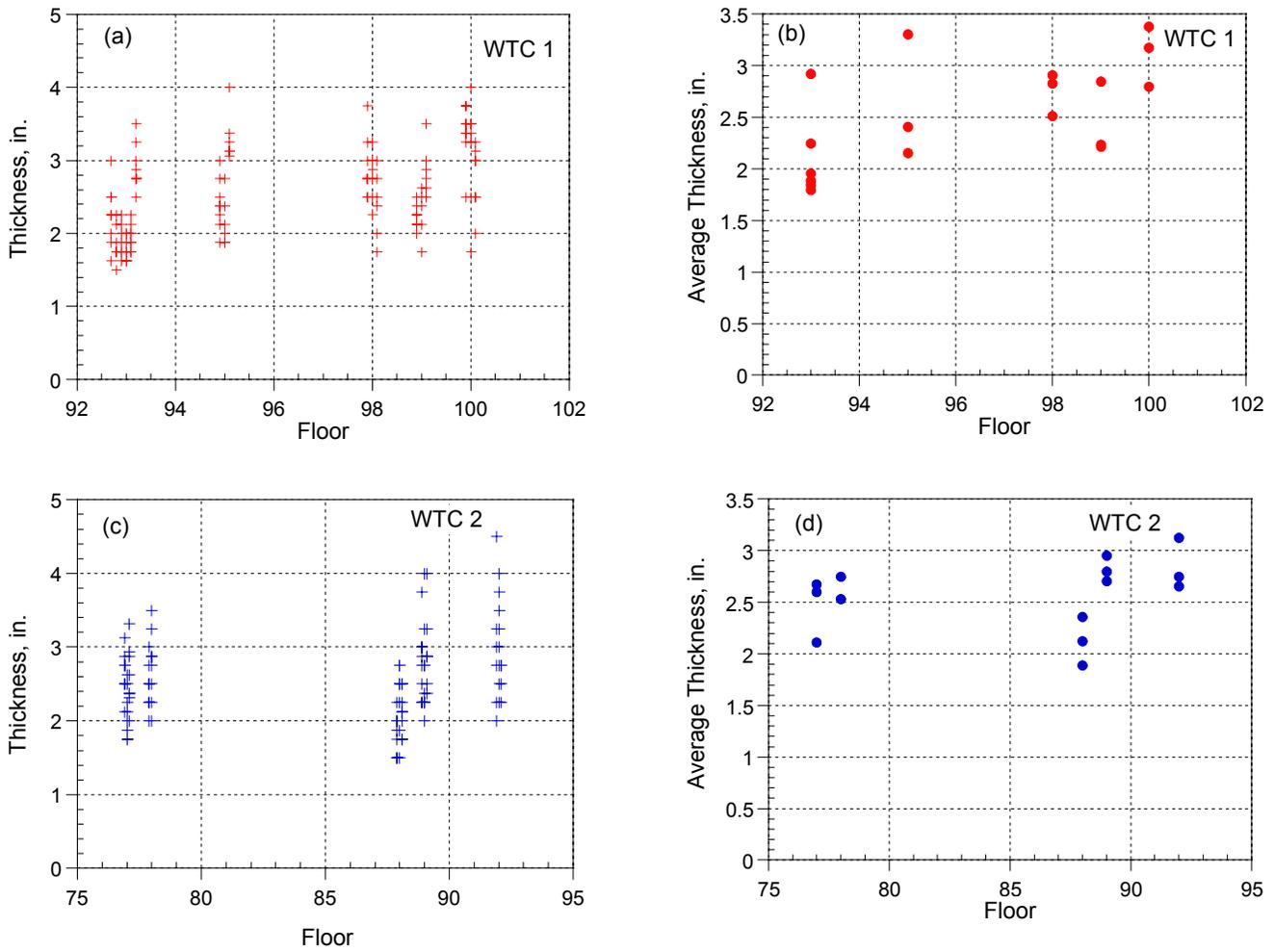
**Figure 4–5. SFRM thickness on floor trusses in upgraded portions of WTC towers: (a) individual measurements in WTC 1, (b) average thickness in WTC 1, (c) individual measurements in WTC 2, and (d) average thickness in WTC 2.**
