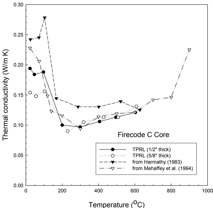
**Figure 6–11. Comparison of the thermal conductivity measurements from TPRL with other literature values for Firecode C Core gypsum panel.**
