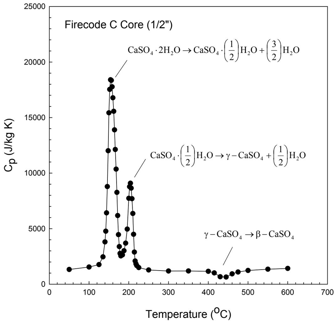
Figure B-2. Specific heat capacity of Firecode C Core 1/2 in. gypsum.
