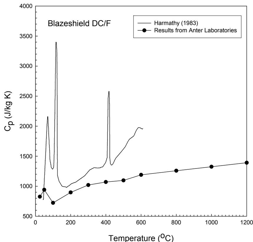
**Figure 6–5. Comparison of BLAZE-SHIELD DC/F specific heat capacity measurements from Harmathy (1983) with present results from Anter Laboratories.**
