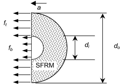
**Figure 7–29. Derivation of acceleration to dislodge SFRM surrounding a round bar.**
