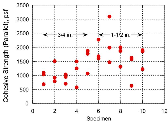
**Figure 7–19. In-plane cohesive strength for BLAZE-SHIELD DC/F specimens.**
