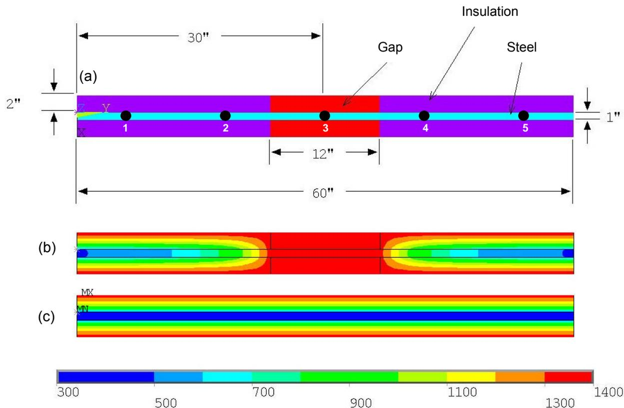
**Figure 5–5. Effects of gap in fire-resistive material: (a) model of plate with SFRM having 2 in. uniform thickness and 12 in. gap, (b) isotherms (K) at time = 50 min with 12 in. gap, and (c) isotherms without gap.**
