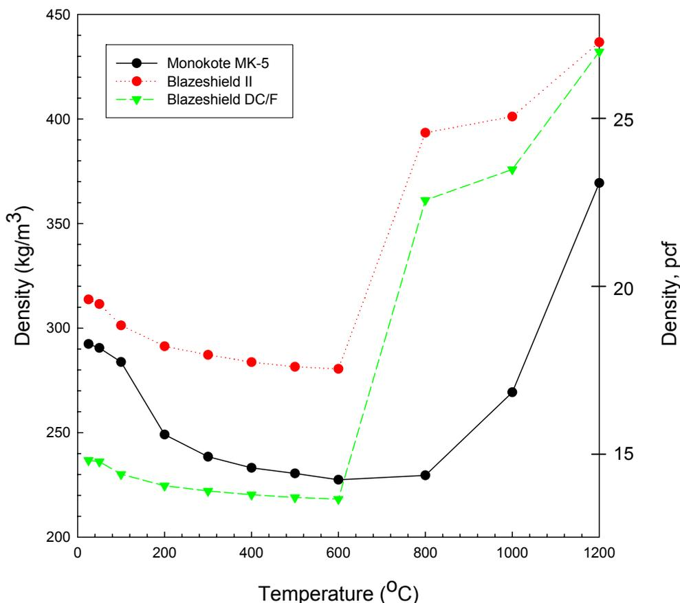
Figure 6–8. Bulk densities of the three SFRMs as a function of temperature.
