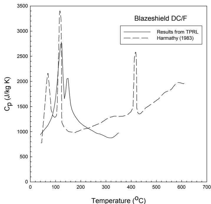
**Figure 6–7. Comparison of specific heat capacity measurements for BLAZE-SHIELD DC/F from TPRL with the results from Harmathy (1983).**
