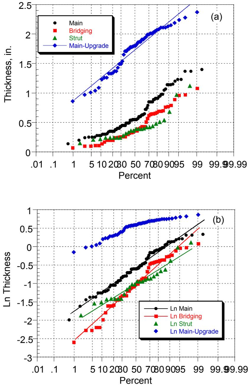
**Figure 4–3. (a) Normal probability plot of estimated SFRM thickness based on photographs, and (b) normal probability plot of natural logarithms of thickness.**
