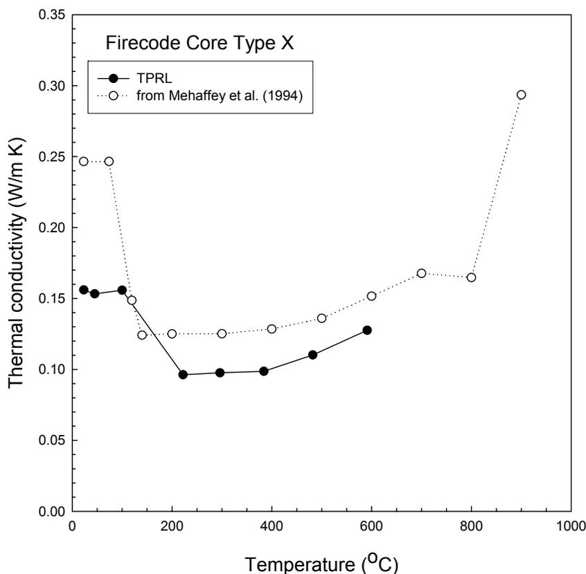
**Figure 6–10. Comparison of the thermal conductivity measurements from TPRL with the data from Mehaffey et al. (1994) for Firecode Core Type X gypsum panel.**
