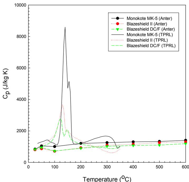
**Figure 6–6. Comparison of specific heat capacity measurements from TPRL with results from Anter Laboratories.**
