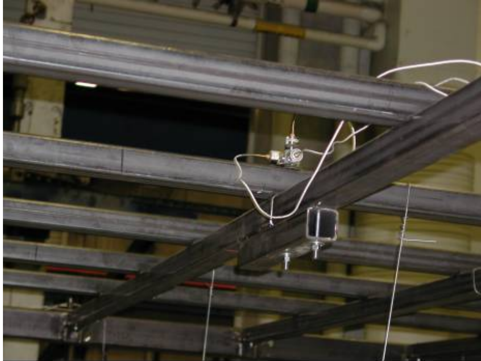
Figure 2–12a. Accelerometers monitoring the response of the test assembly in the center at the top of the test frame.
