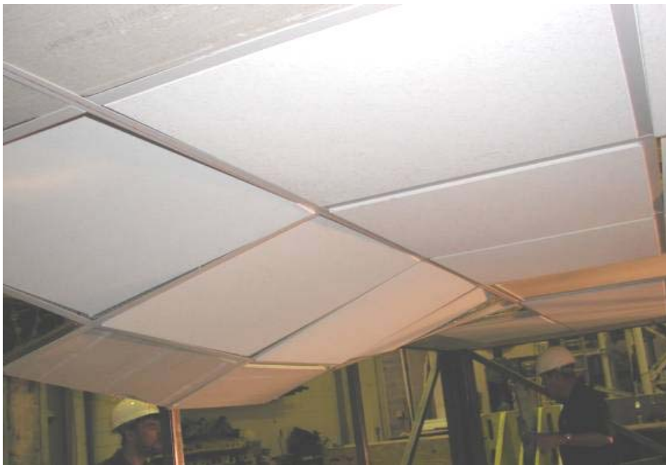
Figure 3–11. Damage to the northern perimeter of ceiling system CS4 following Test 23.
