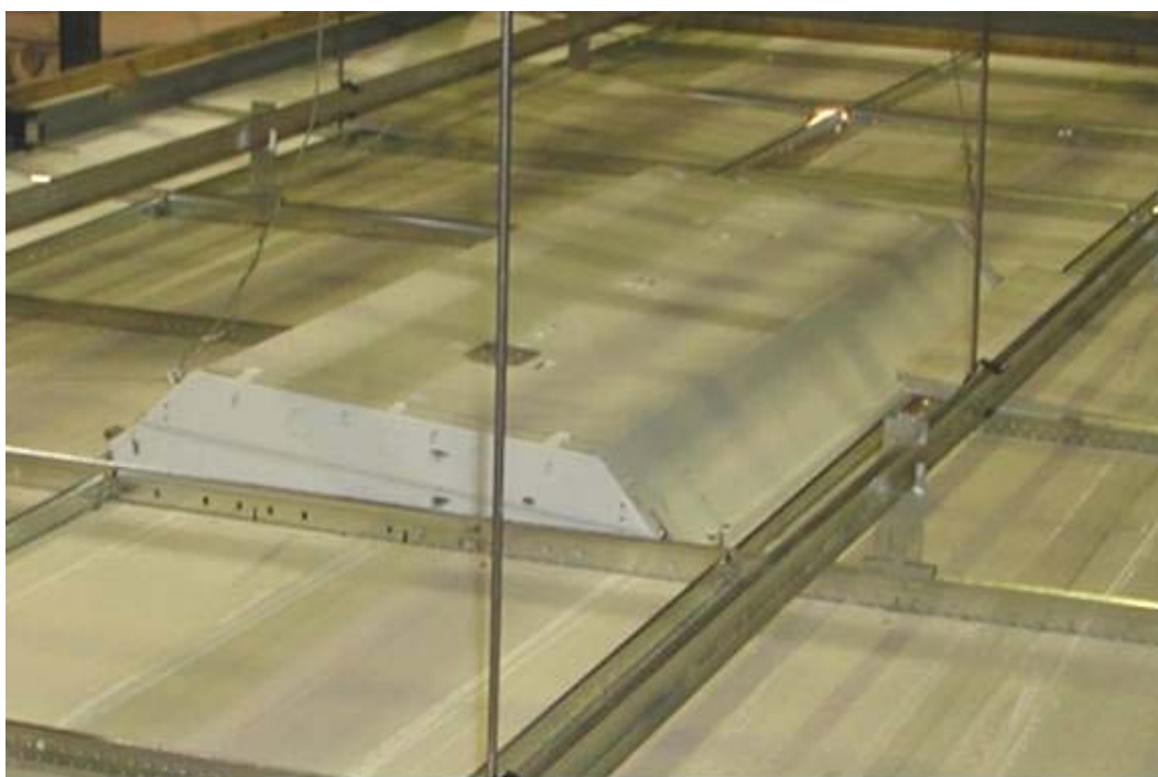
Figure 3–7. Dislodged southern light fixture corner in ceiling system CS2 following Test 14.
