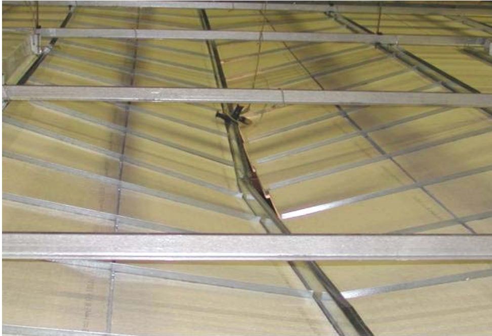
Figure 3–10. Damage to the center of ceiling system CS3 following Test 23.
