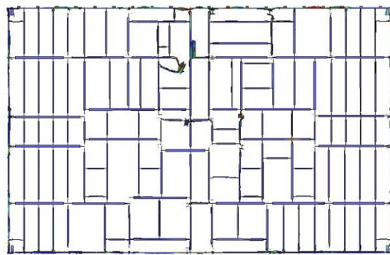
(a) Floor 93 core framing damage
