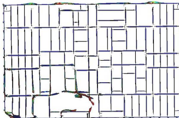
(c) Floor 79 core framing damage
