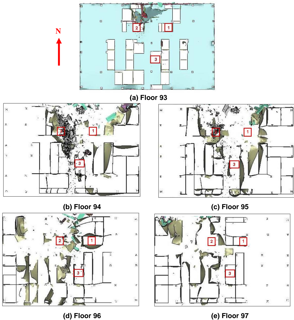
Figure 9-124. Base case stairwell disruption in WTC 1.
