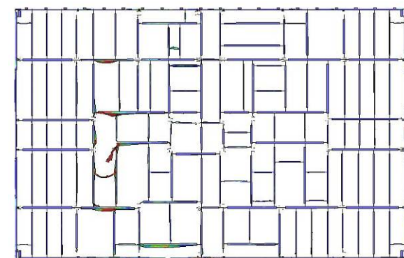
(f) Floor 98 core framing damage
