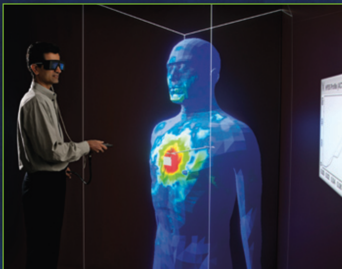
Electronics engineer Kamran Sayrafian uses NIST's Reconfigurable 3D Immersive Platform to study and model how radio frequency (RF) waves propagate through the human body. This research is being used to support the development of standards for implantable and wearable wireless medical devices. © Nicholas McIntosh
