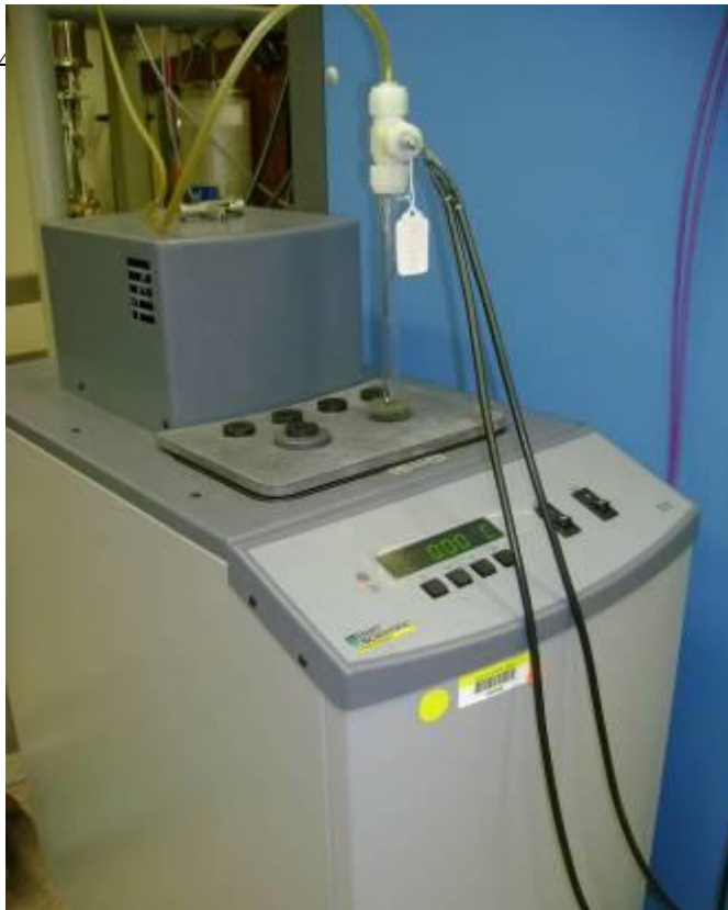
Figure 4.5. The WTP cell maintenance bath with a glass adapter probe installed in a WTP cell.
