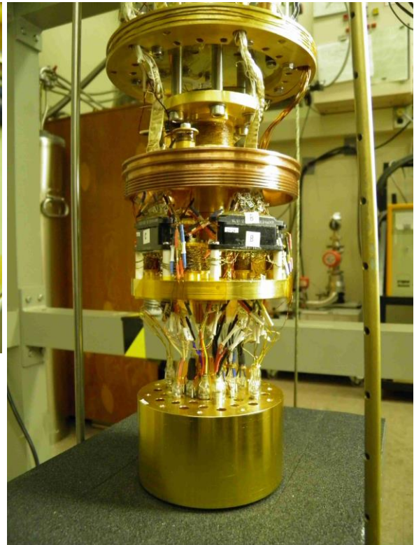
Figure 5.3 The 3 He cryostat with a large comparison block installed.
