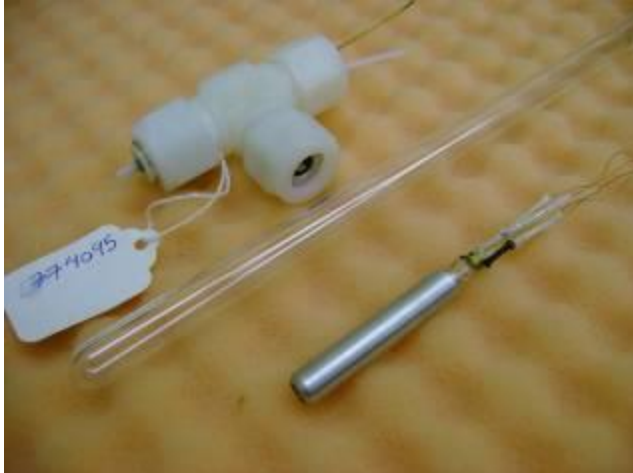
Figure 4.4 The adapter probe assembly showing a capsule SPRT installed in an aluminum bushing.
