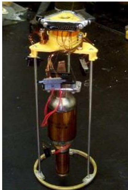
Figure 4.1 A Sealed Triple Point Cell shown suspended in a frame for calorimetric triple point realizations.
