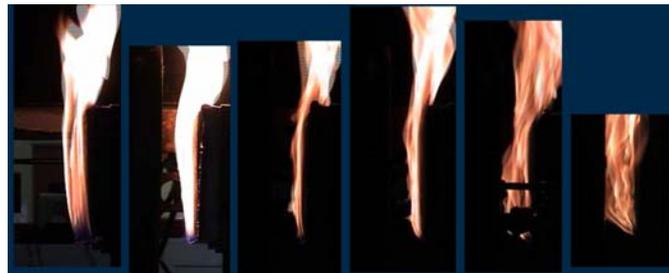
**Figure 6 - Experimental flame images of PMMA samples burning in the vertical configuration for (0, 5, 10, 25, 50, and 75) kW/m<sup>2</sup>.**
