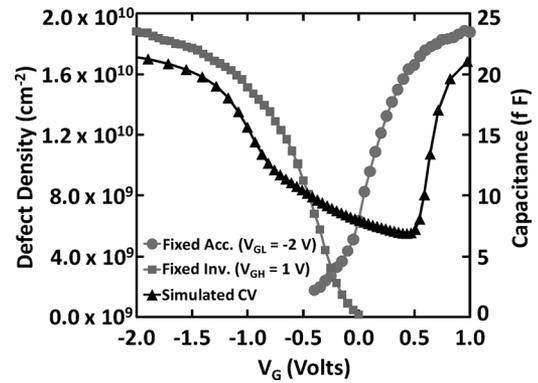
FIG. 2.  $I_{CP}$  normalized to defect density versus pulse height for the cases of fixed accumulation and fixed inversion providing a count of defects as a function of energy. Also included is a simulated CV curve.
