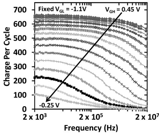
FIG. 1. The effect of insufficient interface trap filling time is illustrated by plotting charge per cycle versus CP frequency for the case of fixed accumulation. Clearly, as  $V_{GH}$  is reduced from inversion deep into depletion or the frequency is increased, an apparent loss in charge per cycle occurs. This effect must be avoided.
