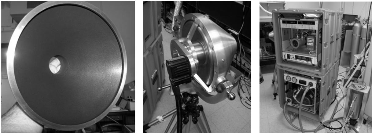
**Figure 2.** Inside of the optical cavity showing the black coating (left), front view of the BB Prime (center), and portable, modular control equipment (right).
