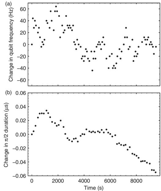
FIG. 3. Changes in (a) qubit transition frequency and (b)  $\pi/2$  duration during the benchmarking experiments. Change is defined as the difference between the recalibrated value and the first calibration. Typical transition frequencies and  $\pi/2$  durations are approximately 1.250 7385 GHz and 20.50  $\mu\text{s}$ , respectively.
