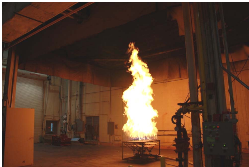
Figure 1. Photograph of natural gas burner operating at 8 MW.
