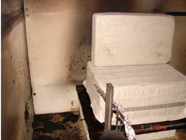
Figure 2. Flaming ignition of a chair mockup. The ignitor was removed after 40 s.
