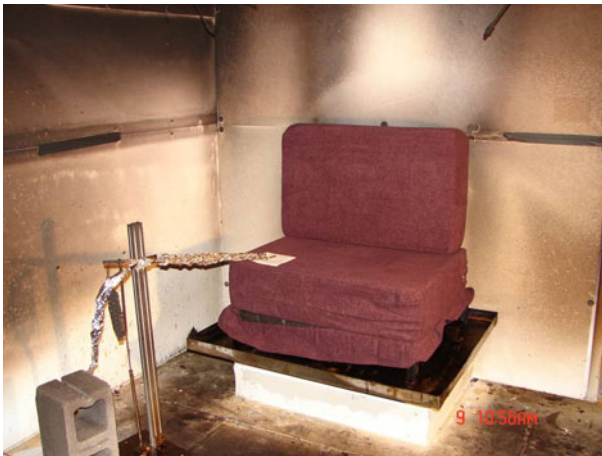
Figure 3. Smoldering ignition of a chair mock-up. The heat source was removed after smoldering initiation (about 6 min).
